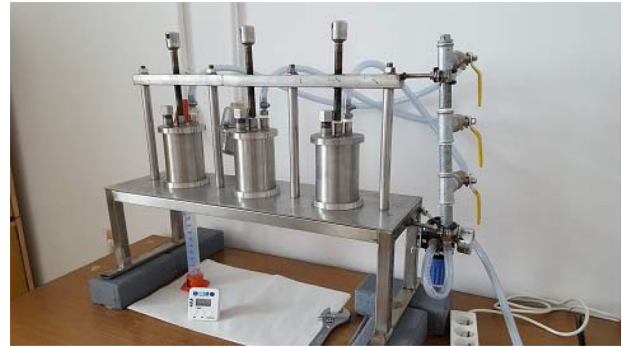
Fig. 2. Pressure filtration station.
