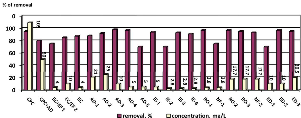
Fig. 1. Efficiency of fluoride removal by different technologies. CPC, precipitation/coagulation; EC, electrocoagulation; AD, adsorption; EF, electroflotation; IE, ion-exchange; RO, reverse osmosis; NF, nanofiltration and ED, electrodialysis.
