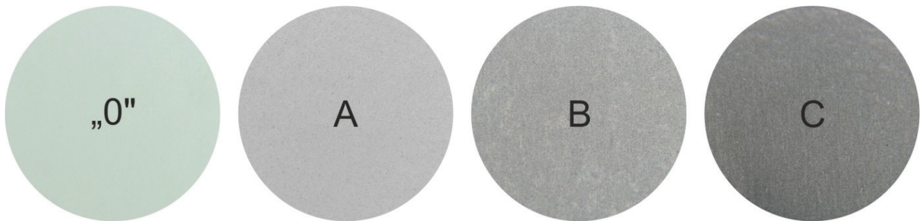
Fig. 1. Images of membrane “0” (pure PAN) and MWCNT/PAN composite membranes.
