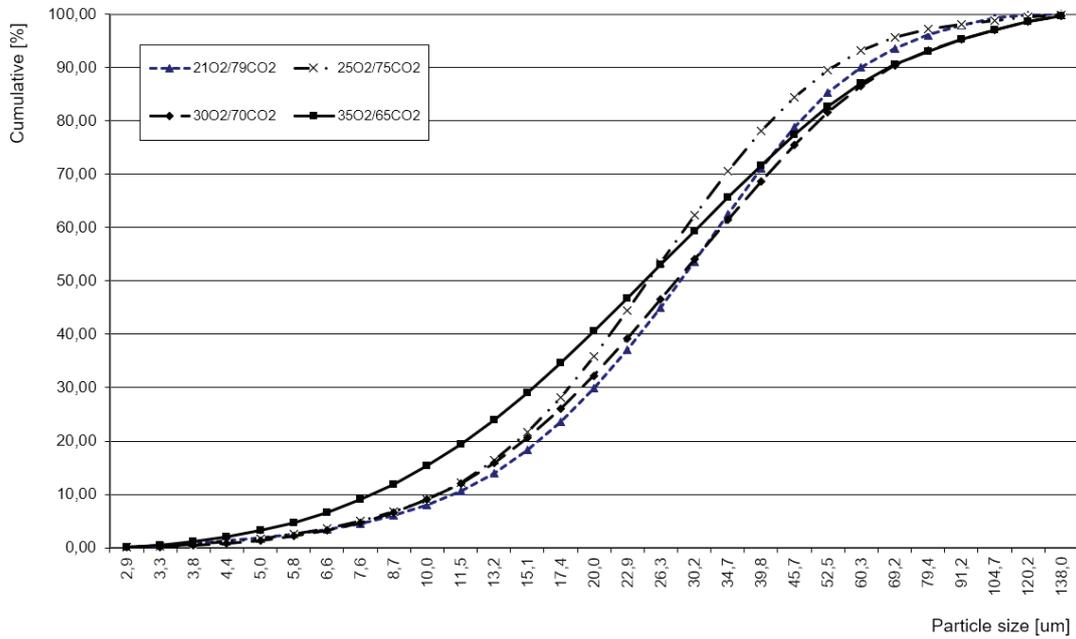
Fig. 2. Particle size distribution of FSC30 fly ash obtained in different atmospheres.
