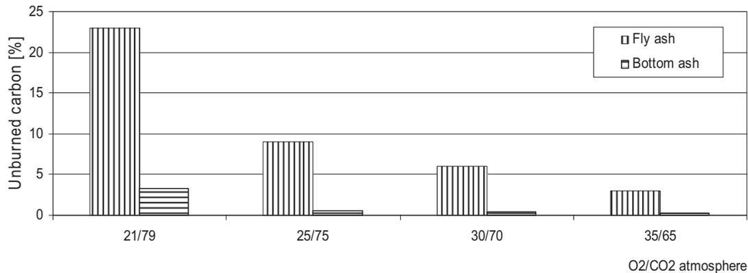
Fig. 1. Mass fraction of unburned carbon in fly and bottom ash.
