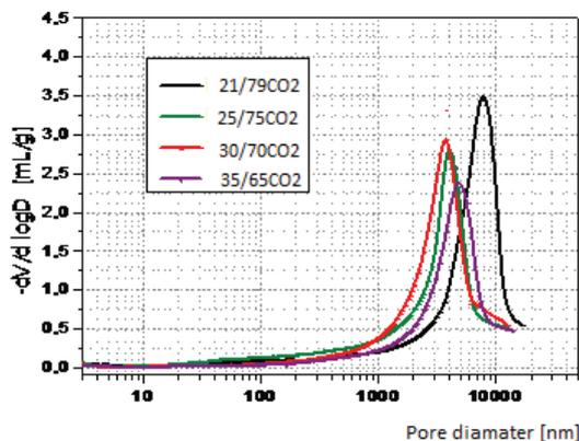
Fig. 4. Pore volume distribution of FSC30 fly ash.
