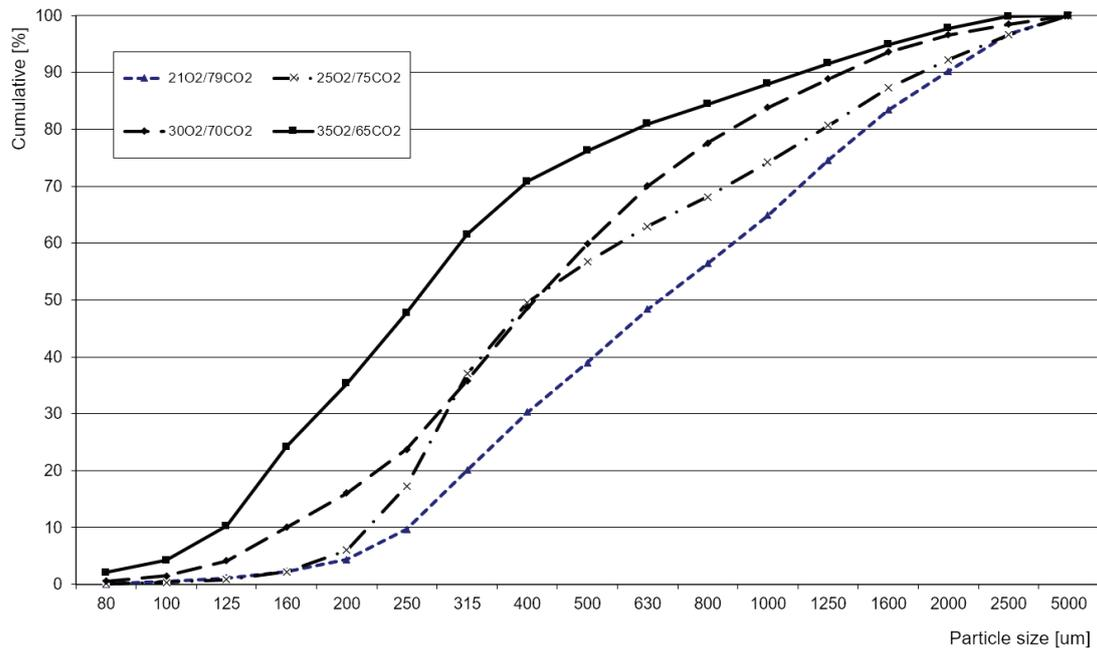
Fig. 3. Particle size distribution of FSC30 bottom ash obtained in different atmospheres.
