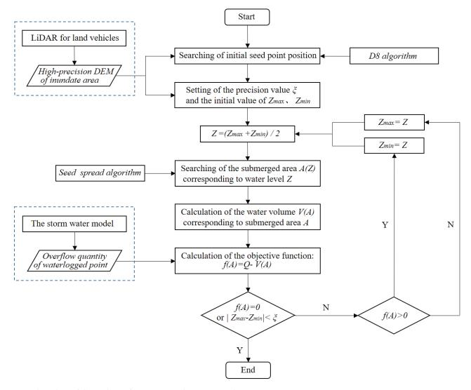
Fig. 4. Flow chart of the analysis of water accumulation in inundate area.
