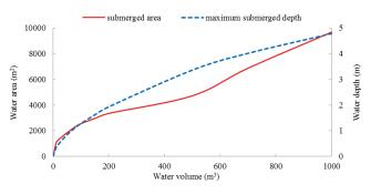
Fig. 8. The relation curves of water volume and submerged features of the studied inundate area.
