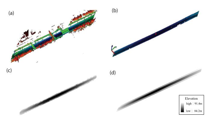
Fig. 5. Generation process of the DEM data in the studied inundate area: (a) point cloud row data, (b) point cloud edited data of pavement, (c) generated DEM data after projection, and (d) DEM edited data.
