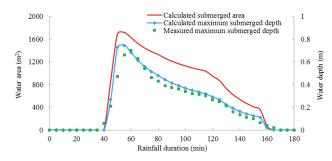
Fig. 10. Comparison between the calculated results and the measured results of submerged information.
