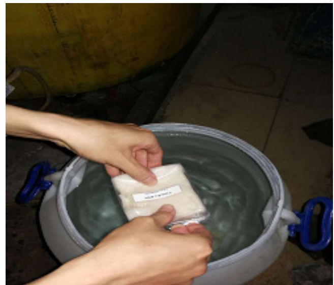
Fig. 9. Operator dissolving the tablet, CrestoPro R594, in the product water.
