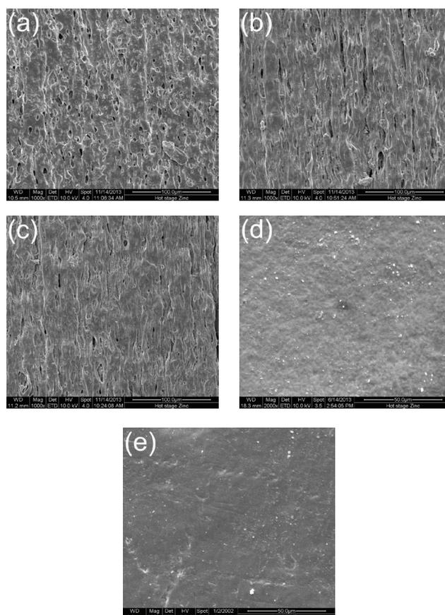
Fig. 4. Outer surface morphologies of PVC hollow fiber matrix membrane and HR PVC hollow fiber membranes. (a) M0, (b) M1, (c) M2, (d) M1-1, (e) M2-1.
