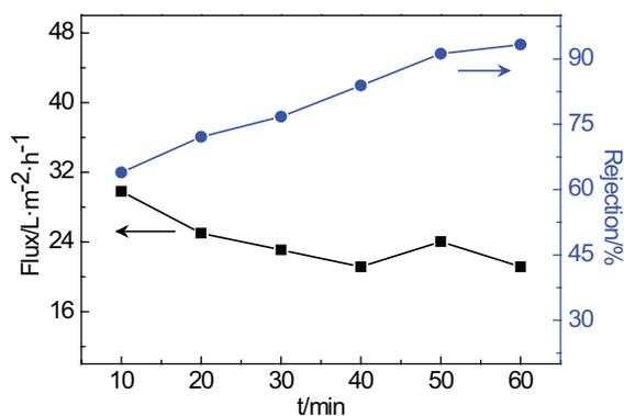
Fig. 9. Variation of permeate flux and rejection rate with time. (M2-1, operating pressure: 0.1 MPa, testing temperature: 20°C).
