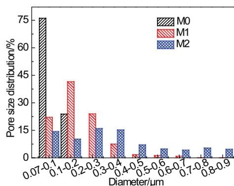
Fig. 7. Pore size distribution of PVC hollow fiber matrix membrane.
