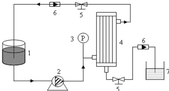
Fig. 2. Schematic diagram of filtration system: (1) feed tank, (2) feed pump, (3) manometer, (4) membrane cell, (5) control valve, (6) rotameter, (7) permeate tank.
