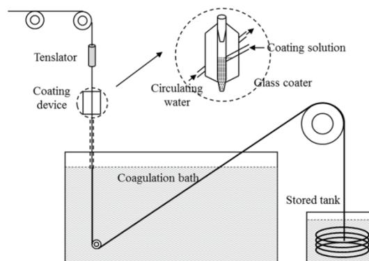
Fig. 1. Schematic diagram of the preparation system.
