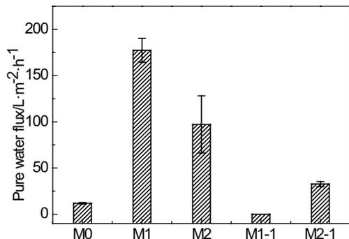
Fig. 8. Pure water flux of prepared PVC matrix and HR PVC hollow fiber membranes.
