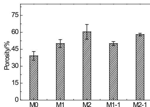
Fig. 6. Porosity of prepared PVC matrix and HR PVC hollow fiber membranes.
