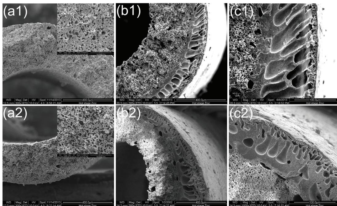
Fig. 3. Cross-section morphologies of PVC hollow fiber matrix membrane and HR PVC hollow fiber membranes. ((a1) M1, (b1) and (c1) M1-1, (a2) M2, (b2) and (c2) M2-1).
