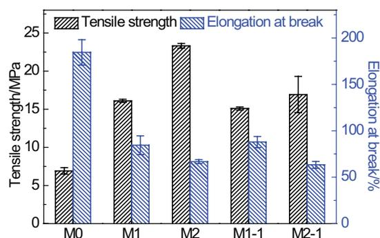
Fig. 5. Mechanical properties of prepared PVC matrix and HR PVC hollow fiber membranes.
