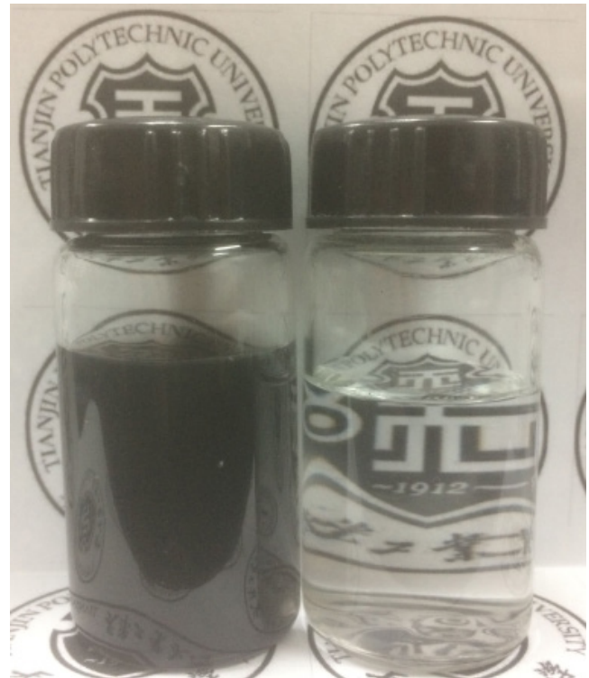
Fig. S7. The feed solution and filtrate solution filtered by 20P(50C50G) membrane formed in 20 °C air bath
