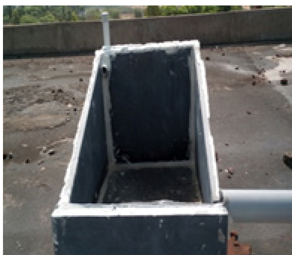
Fig. 4. Solar still with sensible heat materials.
