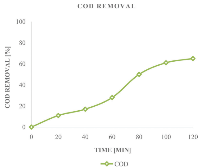
Fig. 12. COD removal of safranin solution for UV/H 2 O 2 /Fe-RHA ( C_{o(SAF)} = 15 mg/L; pH = 3.0; catalyst dose = 0.1 g; T = 30^{\circ}\text{C} ; H 2 O 2 = 8 mM; V = 100 mL).
