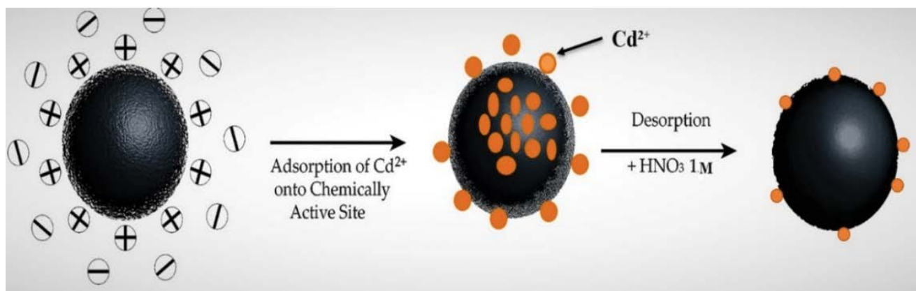
Fig. 10. Schematic illustrations of adsorption–desorption of Cd(II) ions onto the surface of PEFA.
