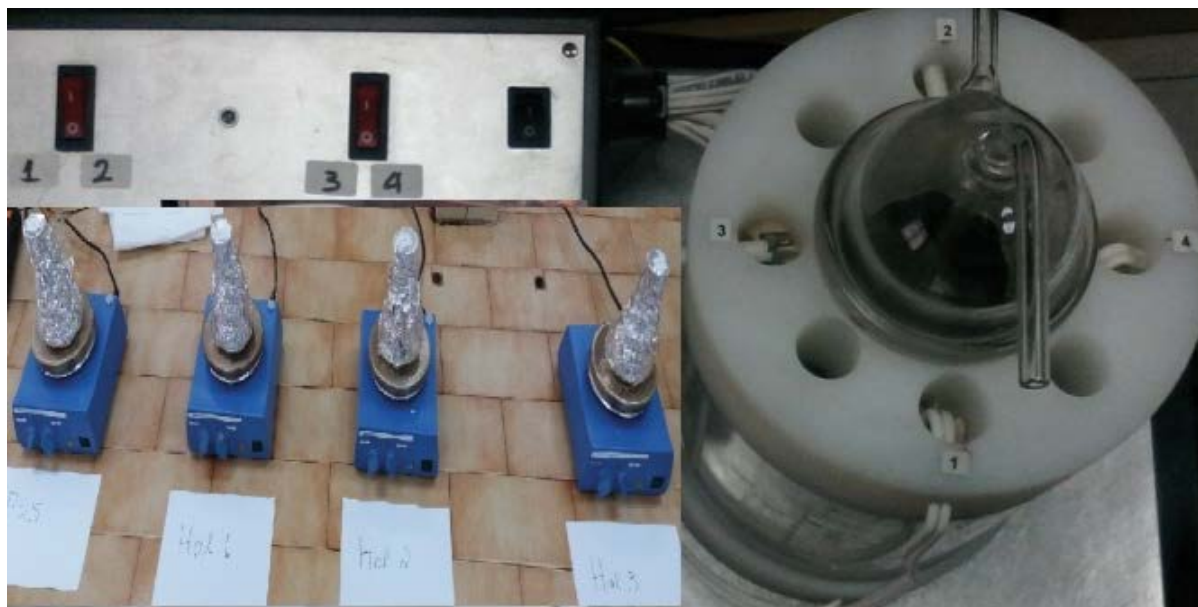
Fig. 1. Photographs showing the samples preparation and photocatalytic reactor used in all experiments.
