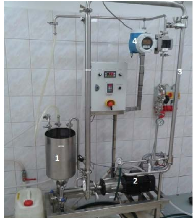
Fig. 1. Laboratory UF unit with a tubular ceramic membrane: 1 – feed tank, 2 – pump, 3 – tubular ceramic membrane, and 4 – flowmeter.
