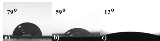
Fig. 3. Contact angle versus the method of GO location into the membrane: (a) without GO, (b) mixing with the polymer, and (c) applied via spraying.
