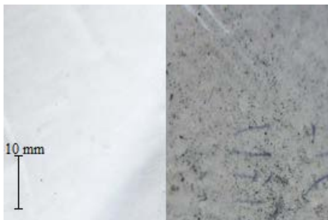
Fig. 1. Unmodified membrane (L) and membrane modified with CNTs (R).
