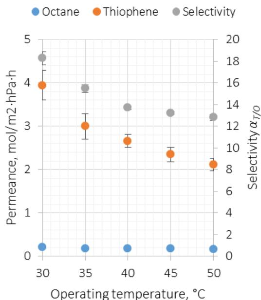
Fig. 7. The impact of operating temperature on thiophene and octane permeances at thiophene feed concentration of 0.07 wt. % and permeate pressure of 100 Pa.
