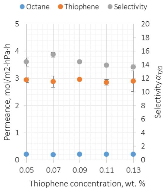
Fig. 10. The influence of thiophene concentration in feed on thiophene and octane permeances and selectivity at temperature of 35°C and permeate pressure of 100 Pa.
