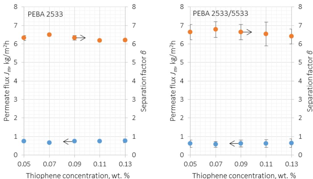
Fig. 8. The influence of thiophene concentration in feed on the total permeate flux and separation factor at temperature of 35°C and permeate pressure of 100 Pa.
