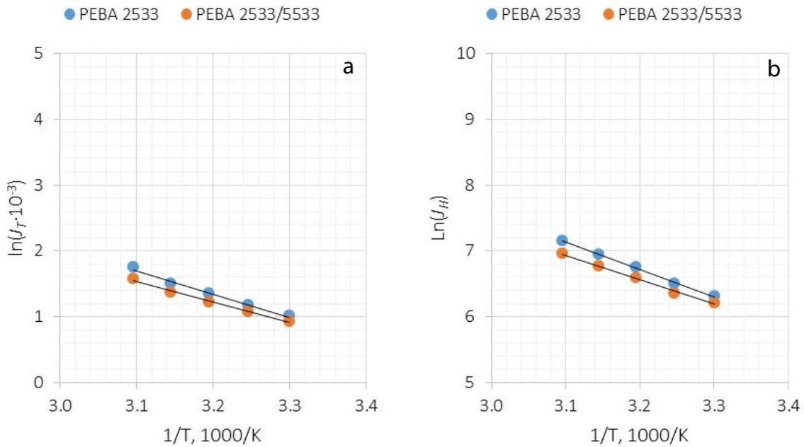
Fig. 6. Arrhenius-type relation on components fluxes for PEBA membrane at feed concentration of 0.07 wt. % and permeate pressure of 100 Pa; (a) thiophene and (b) octane.
