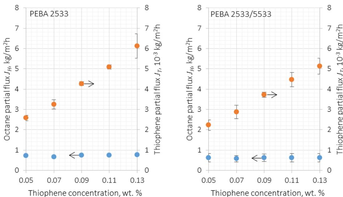
Fig. 9. The influence of thiophene concentration in feed on thiophene and octane partial fluxes at temperature of 35°C and permeate pressure of 100 Pa
