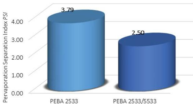
Fig. 11. PSI index values for tested homogenous PEBA membranes.
