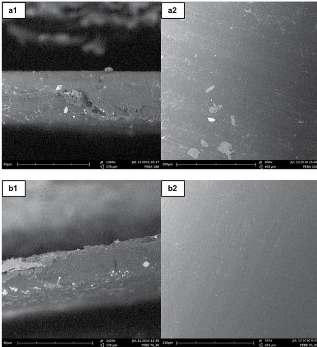
Fig. 2. SEM images of prepared homogeneous membranes: 1 – membrane cross-section; 2 – membrane surface; a – PEBA 2533; b – PEBA 2533/5533.
