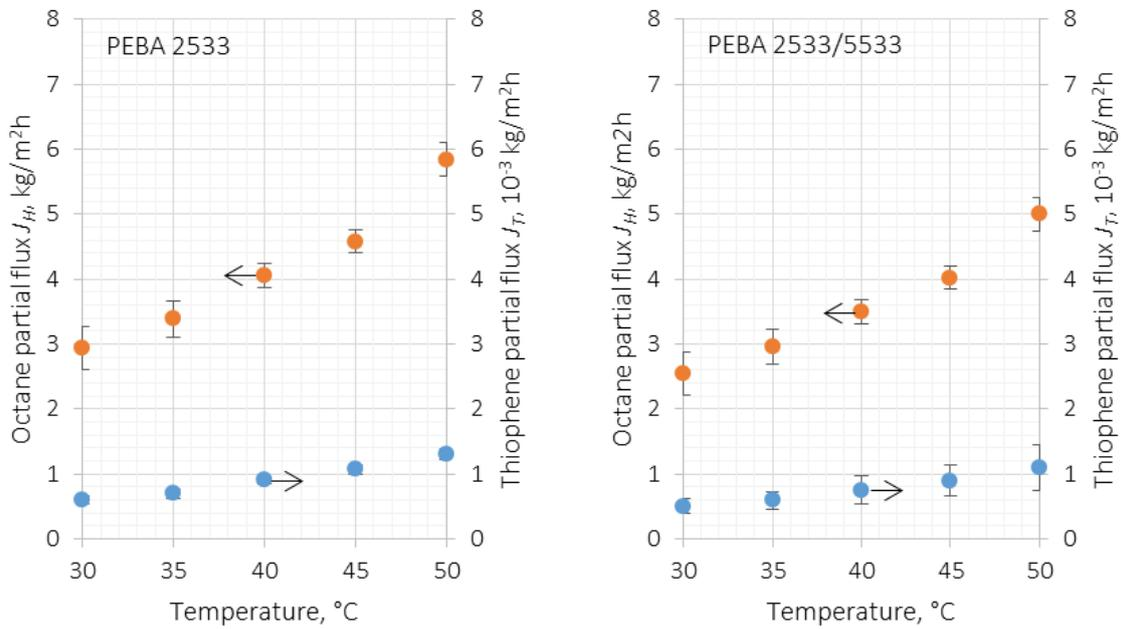
Fig. 5. The impact of operating temperature on the partial fluxes of components at thiophene feed concentration of 0.07 wt. % and permeate pressure of 100 Pa.
