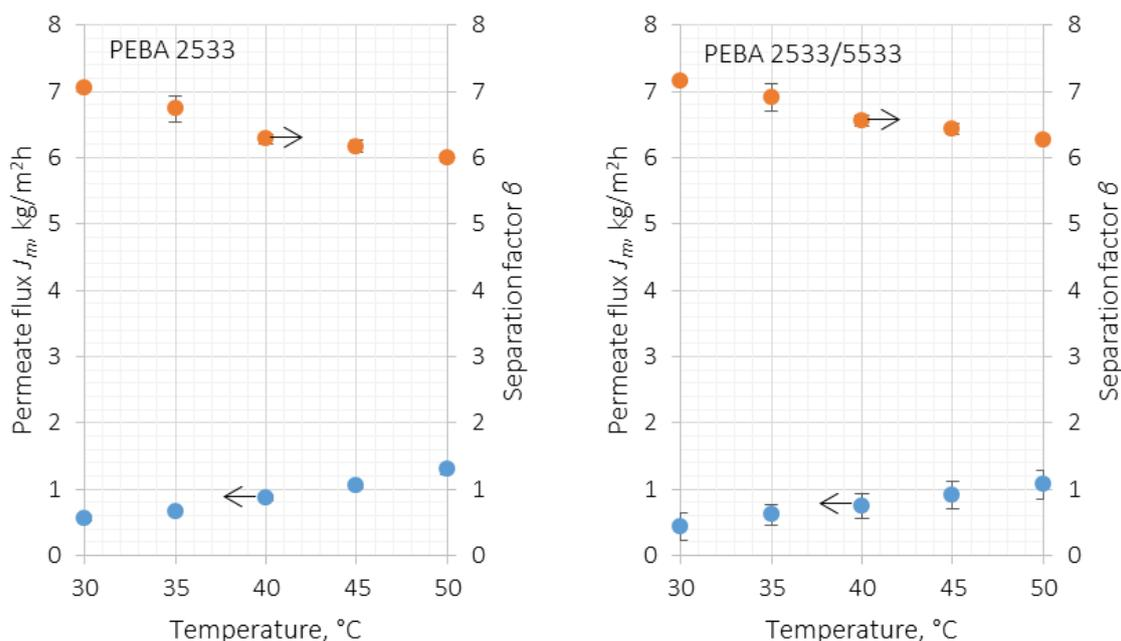
Fig. 4. The impact of operating temperature on the total permeate flux and separation factor at thiophene feed concentration of 0.07 wt. % and permeate pressure of 100 Pa.
