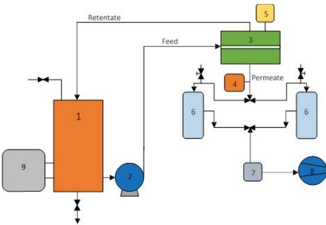
Fig. 3. The scheme of the vacuum pervaporation set-up – 1 – feed tank; 2 – circulation pump; 3 – membrane module; 4 – vacuum gauge; 5 – thermometer; 6 – cooling traps; 7 – buffer tank; 8 – vacuum pump; and 9 – thermostat.
