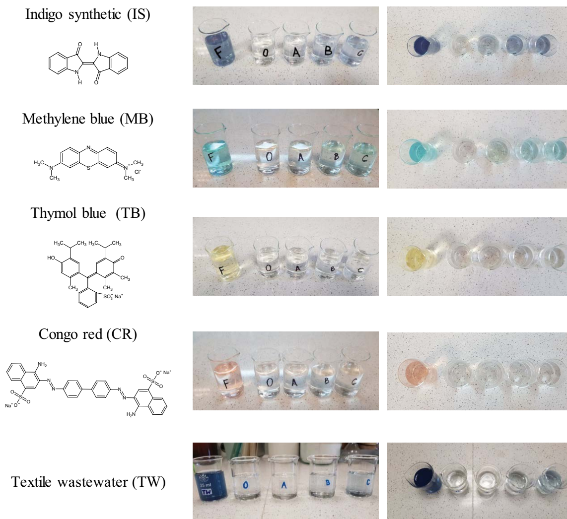
Fig. 4. Photographs of permeates obtained during ultrafiltration of dyes (IS, MB, TB, and CR) and textile wastewater (TW) on individual membranes. Markings: F – feed; 0 – permeate after membrane “0”; A – permeate after membrane A; B – permeate after membrane B; and C – permeate after membrane C.
