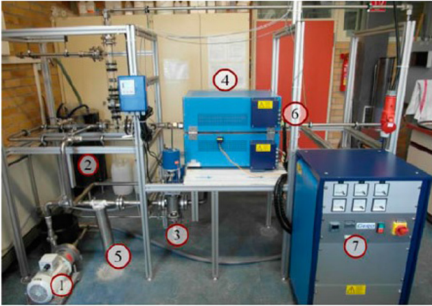
Fig. 4. A photo of the test facility which included: 1) centrifugal pump, 2) supply tank, 3) flow meter, 4) heater, 5) filter, 6) heated section and 7) heater control panel.
