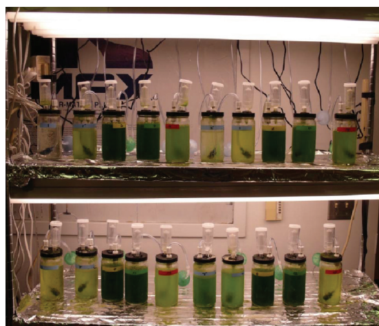
Fig. 1. Experimental setup for studying growth of algae in concentrate, f/2, and 50:50 media.
