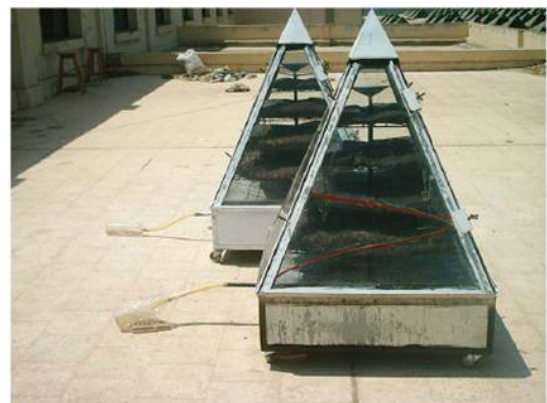
Fig. 3. Photograph of the pyramid desalination system. (Source: Kabeel [28])
