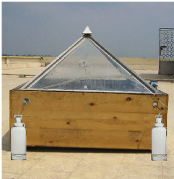
Fig. 5. Photograph of the fabricated concave wick solar still. (Source: Kabeel [29])
