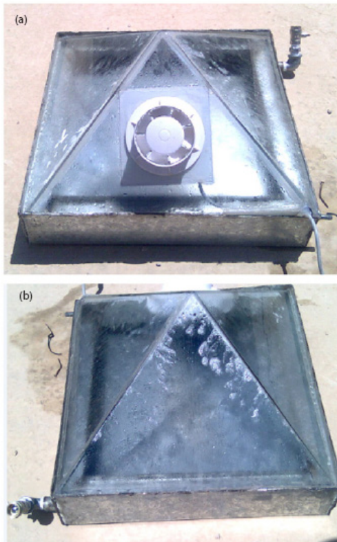
Fig. 14. PSSs (a) with fan and (b) without fan. (Source: Taamneh and Taamneh [40])
