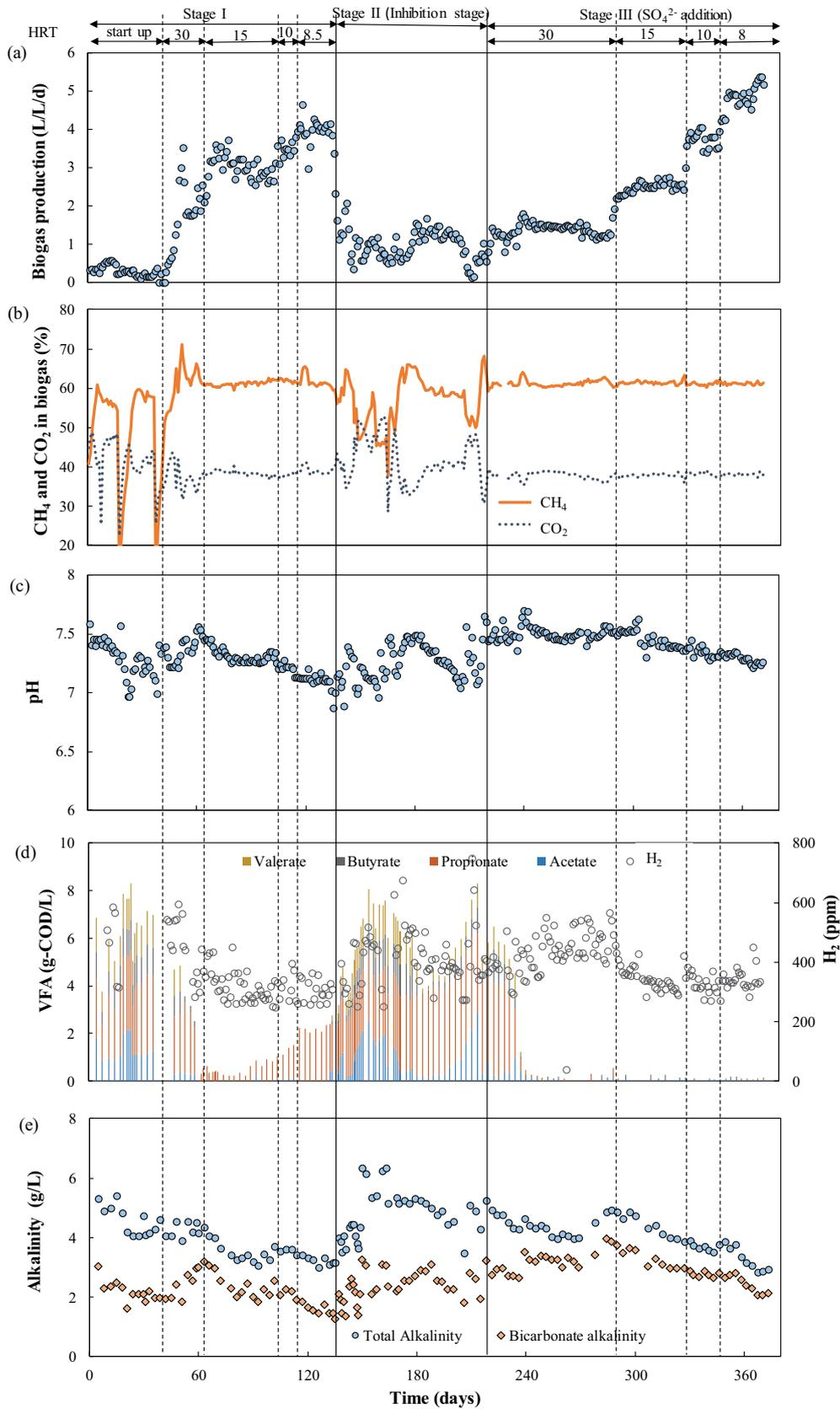
Fig. 2. Performance of the AnMBR reactor during three stages: (a) biogas production; (b) biogas composition; (c) variation in pH; (d) concentration of VFAs and H<sub>2</sub>; and (e) variation in alkalinity and ammonium.
