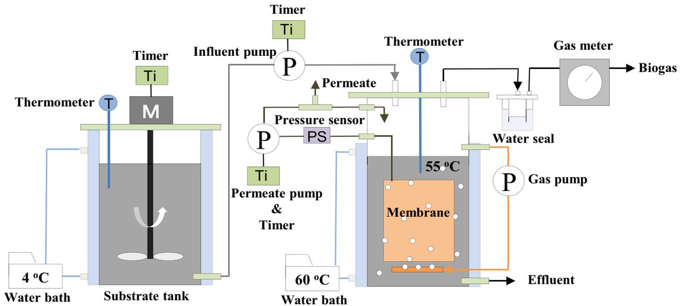
Fig. 1. Thermophilic AnMBR system used in this study.
