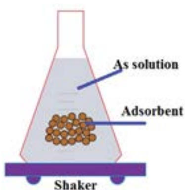
Fig. 2. The scheme of adsorption experiments as a batch method.
