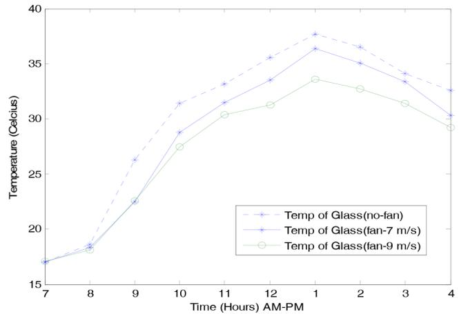
Fig. 5. The effect of fan speed on the glass temperatures in the solar still.
