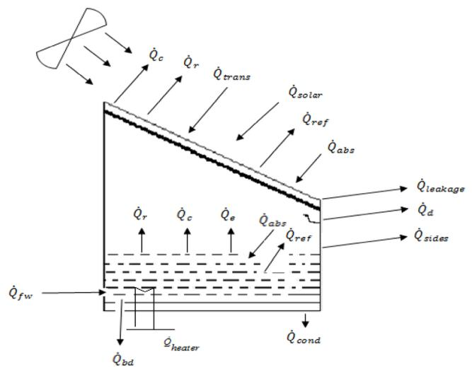
Fig. 1. Various mechanisms of heat transfer in the solar still equipped with a water heater and an external fan.
