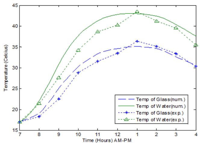
Fig. 11. Comparison of the numerical and the experimental temperature profiles in the solar still using the cooling fan (7 m/s).
