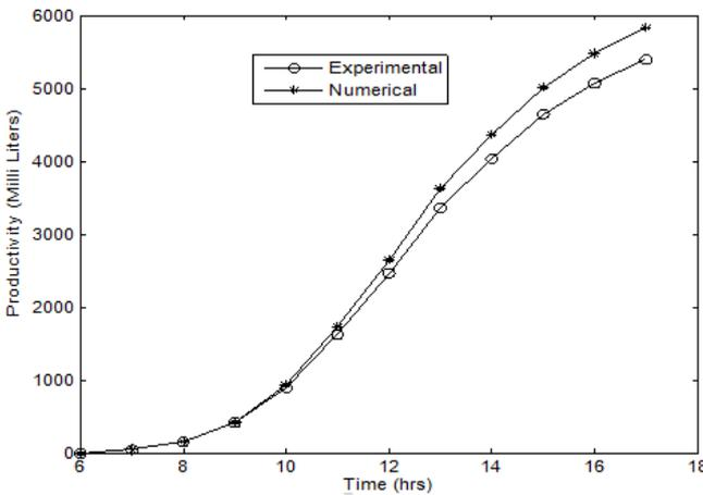
Fig. 13. Comparison of numerical and experimental distilled water production for the solar still with the water heater.
