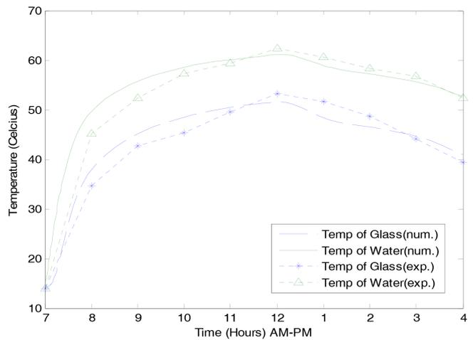
Fig. 10. Comparison of the numerical and the experimental temperature variations in the solar still with water heater.
