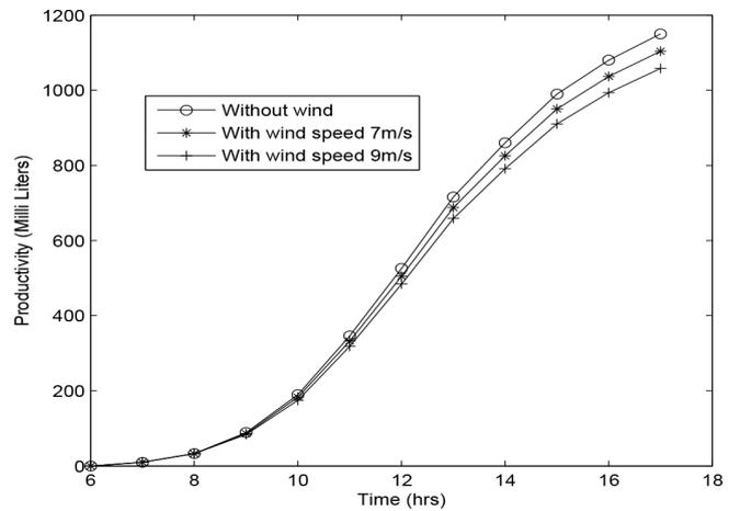
Fig. 7. The effect of the fan speed on the productivity of solar still.
