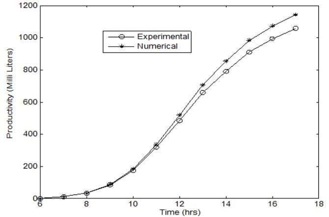
Fig. 15. Comparison of numerical and experimental daily production from the solar still with external fan (9 m/s).
