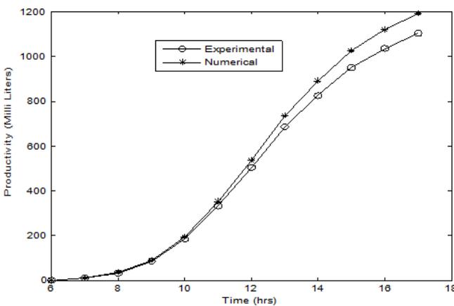
Fig. 14. Comparison of the numerical and the experimental results for the daily production by using external fan (7 m/s)
