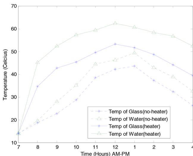
Fig. 3. Temperature measurement in the solar still.
