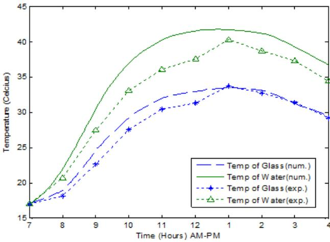
Fig. 12. Comparison of numerical and experimental temperature profiles in the solar still with cooling fan (9 m/s).
