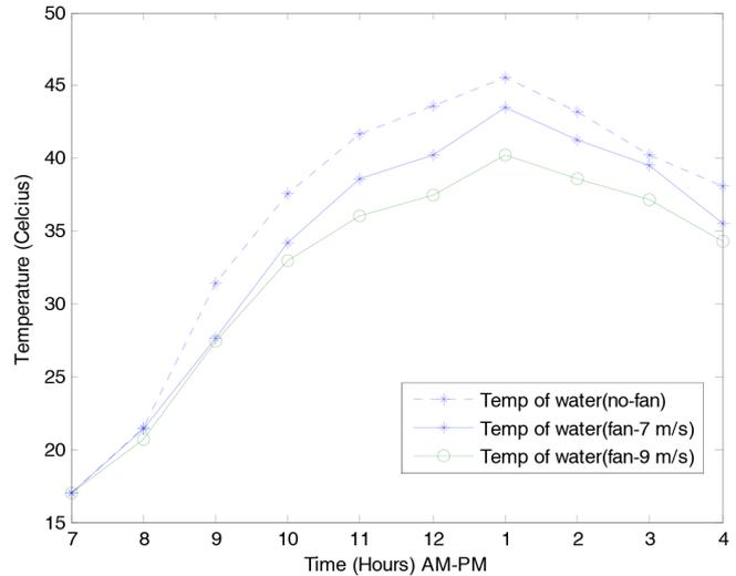
Fig. 6. The effect of fan speed on the water temperatures in the solar still.
