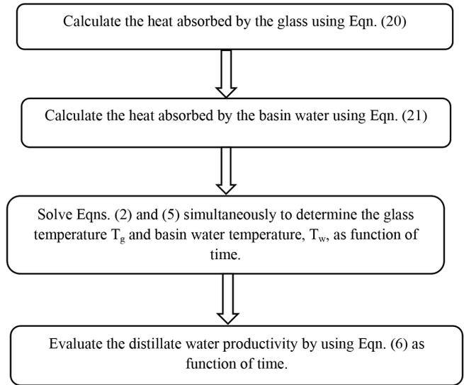
Fig. 9. Flow diagram for the numerical modeling.
