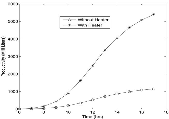
Fig. 4. Distilled water production in the solar still with time.
