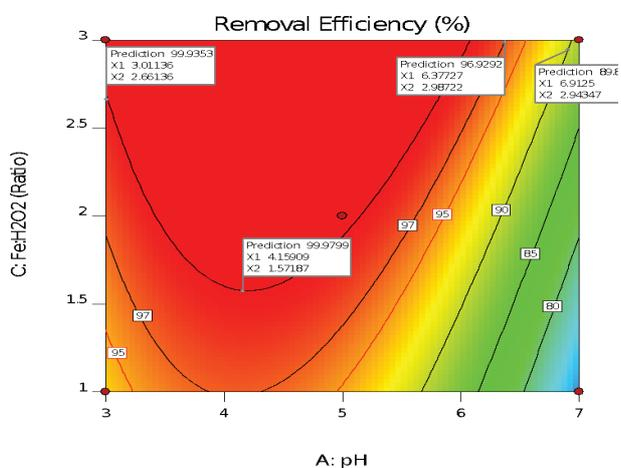
Fig. 3. Contour plot of response surface for acetaminophen removal.
