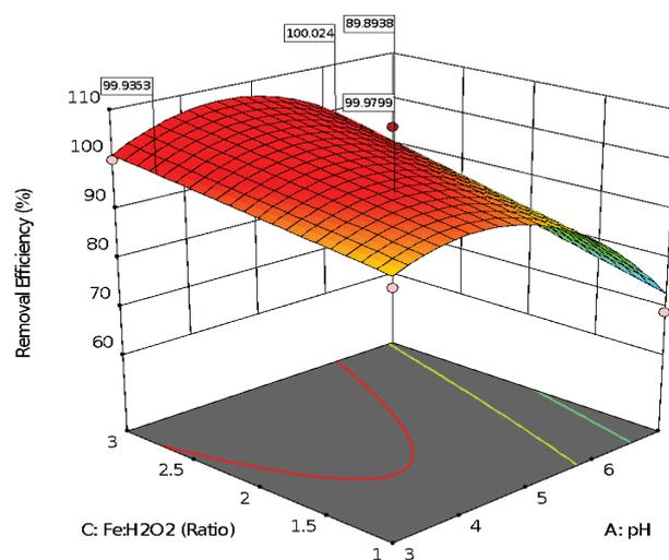
Fig. 4. 3D plot of the response surface of acetaminophen removal.
