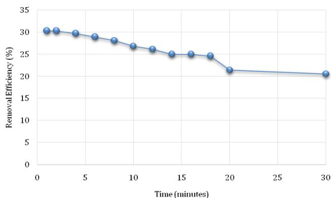
Fig. 7. Adsorptive removal of acetaminophen.
