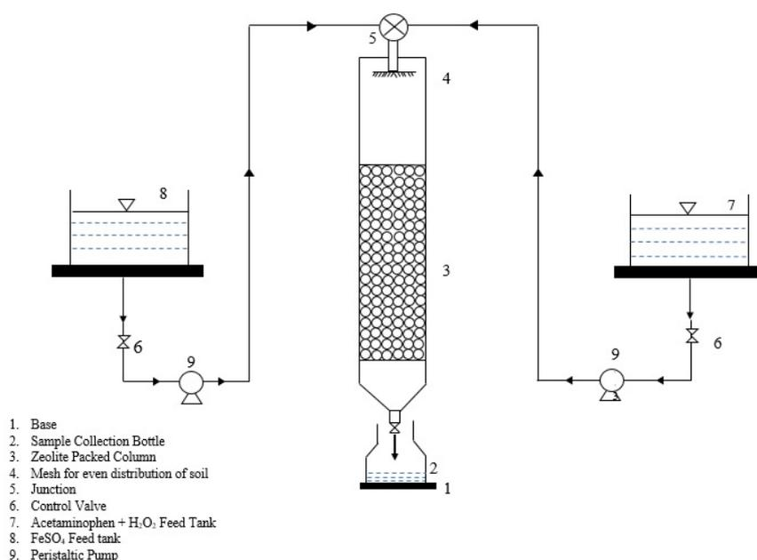
Fig. 1. Schematic diagram of packed column setup for Fenton oxidation.
