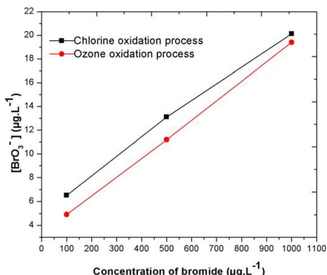
Fig. 2. Effect of initial  $\text{Br}^-$  concentration on bromate formation during chlorination and ozonation process.
