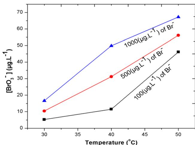
Fig. 5. The formation of bromate during chlorination at various temperatures. (Co: Br<sup>-</sup> 100, 500 and 1000 µg/L).
