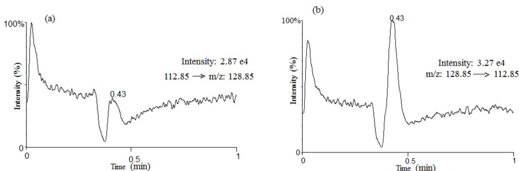
Fig. 6. UPLC–MS/MS chromatograms of BrO<sub>3</sub><sup>-</sup> concentration in commercial bottled water before (a), and after ozonation (b).
