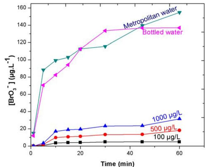
Fig. 4. The formation of bromate with time during ozonation for samples containing 100, 500, and 1000  $\mu\text{g}\cdot\text{l}^{-1}$  of  $\text{Br}^-$ , and metropolitan and bottled water.
