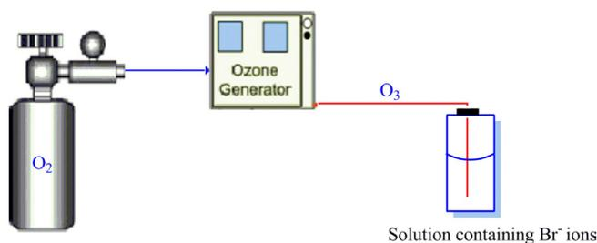
Fig. 1. Schematic system of the ozonation process.
