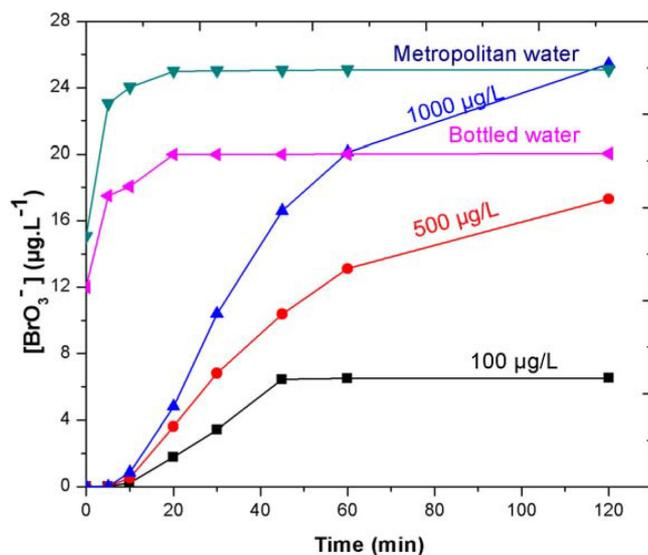
Fig. 3. The formation of bromate with time during chlorination for samples containing 100, 500, and 1000  $\mu\text{g}\cdot\text{l}^{-1}$  of  $\text{Br}^-$ , and metropolitan and bottled water.
