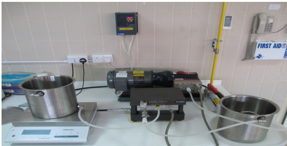
Fig. 3. Schematic figure of the fouling testing unit at DRP.
