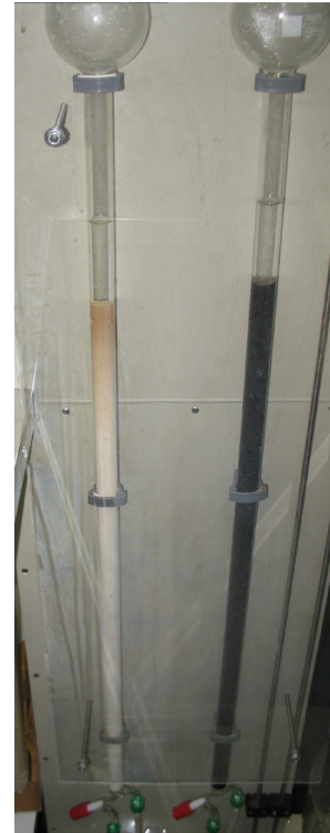
Fig. 4. Lewatit S 5428 resin after five service cycles (left column).
