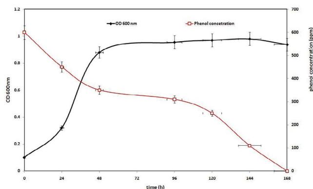
Fig. 4. Growth (as OD 600 nm) and phenol degradation in the culture of *Pseudomonas putida* AHB53P at 30°C in 600 ppm phenol concentrations during 168 h.
