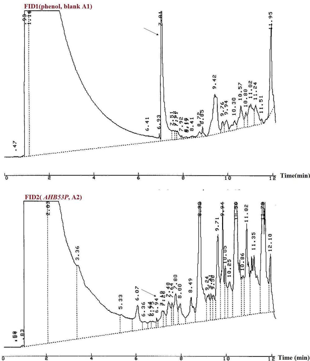
Fig. 7. Analysis of phenol 1,000 ppm by GC after 168 h incubation. FID1 (A1): As blank, and FID2 (B2): By strain AHB53P.
