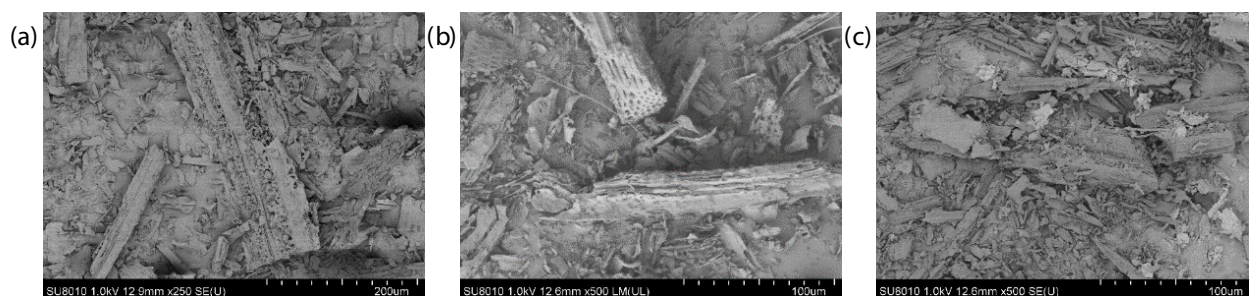
Fig. 3. SEMs of FeBC pyrolyzed at 400^\circ\text{C} (a), 600^\circ\text{C} (b), and 800^\circ\text{C} (c).
