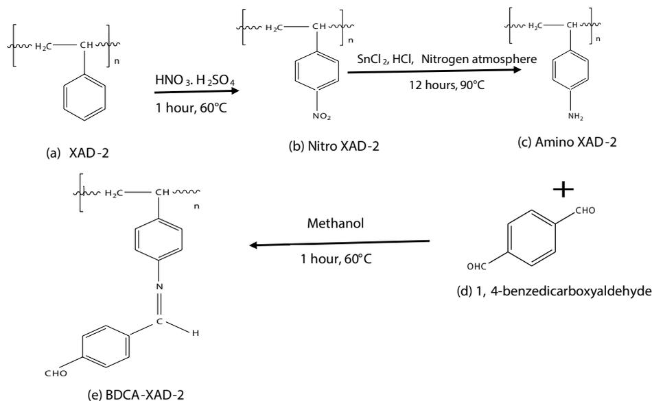
Fig. 1. Reaction scheme for modification of Amberlite XAD-2.
