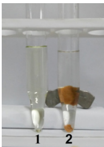
Fig. 10. Magnetic separation of loaded chromate onto CLDH22 ('1', C_i = 55 \text{ mg L}^{-1} and '2', C_f = 4.9 \text{ mg L}^{-1} ).
