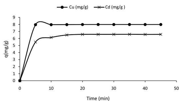
Fig. 4. Effect of time on biosorption of Cu<sup>2+</sup> and Cd<sup>2+</sup> ions on *Bougainvillea spectabilis* (initial conc. = 50 mg/L, dose = 300 mg/50 ml, time = 30 min, pH = 6, stirring speed = 125 rpm).
