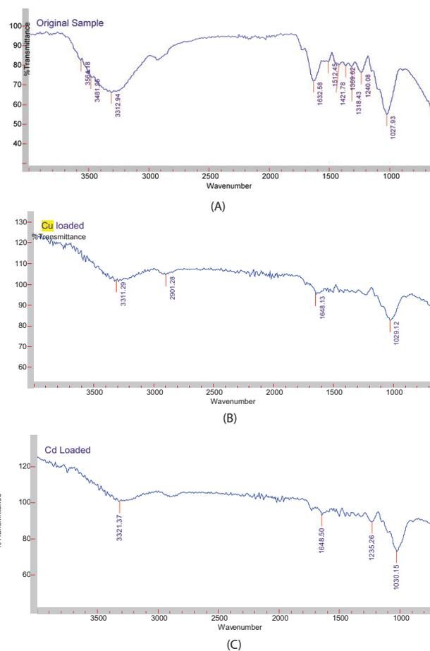
Fig. 1. (a) FTIR spectrum of *Bougainvillea spectabilis* biomass. (b) FTIR spectrum of Copper loaded *Bougainvillea spectabilis* biomass. (c) FTIR spectrum of Cadmium loaded *Bougainvillea spectabilis* biomass.
