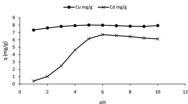
Fig. 3. Effect of pH on biosorption of Cu<sup>2+</sup> and Cd<sup>2+</sup> ions on *Bougainvillea spectabilis* (initial conc. = 50 mg/L, dose = 300 mg/50 ml, time = 30 min, pH = 6, stirring speed = 125 rpm).
