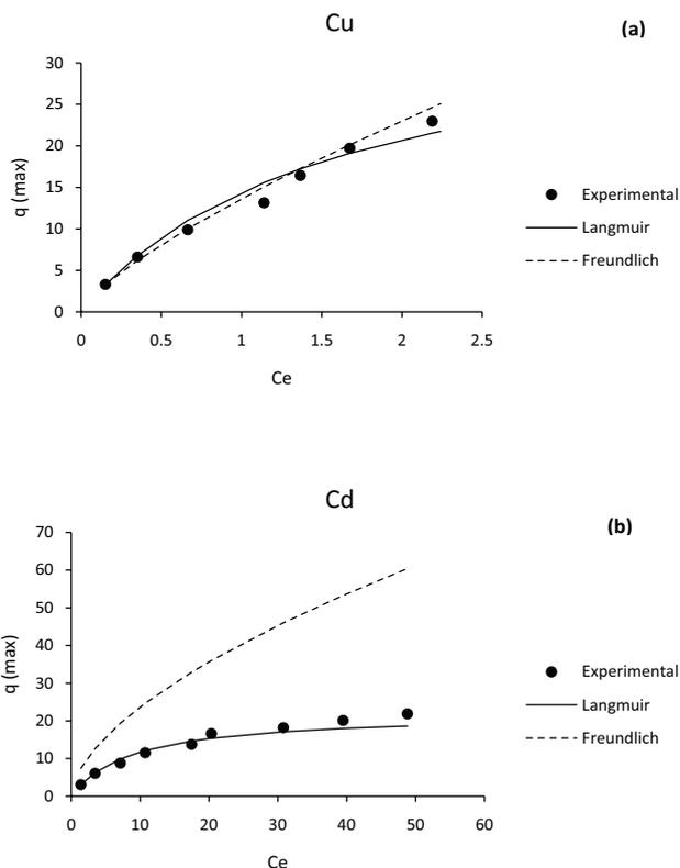
Fig. 6. Non-linear isotherm plots for  $\text{Cu}^{2+}$  (a) and  $\text{Cd}^{2+}$  (b) for Langmuir and Freundlich model.
