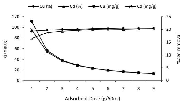
Fig. 2. Effect of *Bougainvillea spectabilis* dose on removal of Cu<sup>2+</sup> and Cd<sup>2+</sup> ions (initial conc. = 50 mg/L, time = 30 min, pH= 6, stirring speed= 125 rpm).
