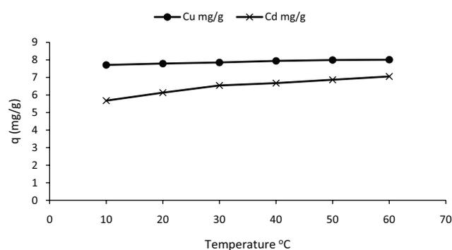
Fig. 5. Effect of temperature on biosorption of Cu<sup>2+</sup> and Cd<sup>2+</sup> ions on *Bougainvillea spectabilis* (initial conc. = 50 mg/L, dose = 300 mg/50 ml, time = 30 min, pH = 6, stirring speed = 125 rpm).
