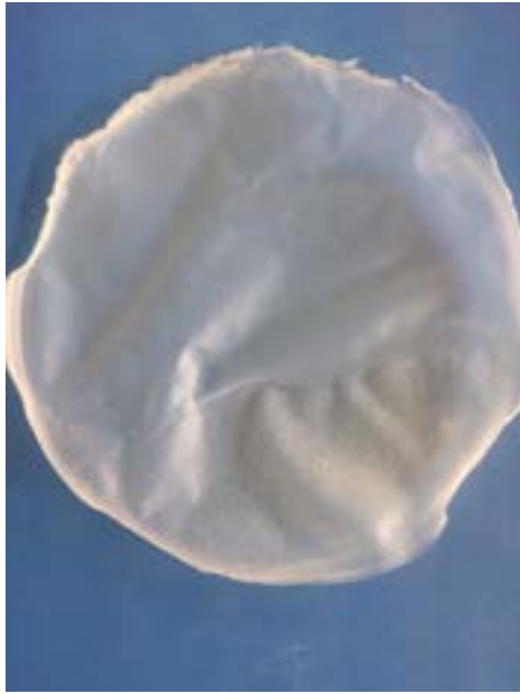
Fig. 1. A representative photo of the film obtained from the three components HAp/HEC/PEG-1000.
