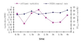
Fig. 7. The effluent turbidity and  $UV_{254}$  removal rate.
