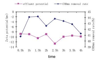
Fig. 8. The effluent Zeta potential and  ${\rm COD}_{\rm Mn}$  removal rate.
