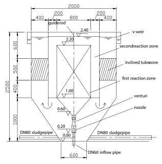
Fig. 1. Structure diagram of micro-vortex clarifier.
