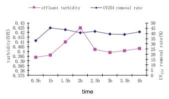
Fig. 5. The effluent turbidity and  $\mbox{UV}_{\mbox{\tiny 254}}$  removal rate.
