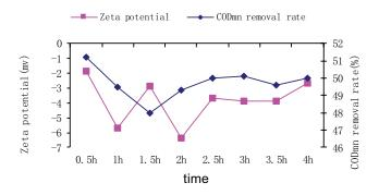
Fig. 4. The effluent Zeta potential and  $COD_{Mn}$  removal rate.
