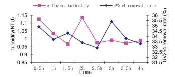
Fig. 3. The effluent turbidity and  $UV_{\rm 254}$  removal rate.
