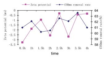
Fig. 6. The effluent Zeta potential and COD<sub>Mp</sub> removal rate.
