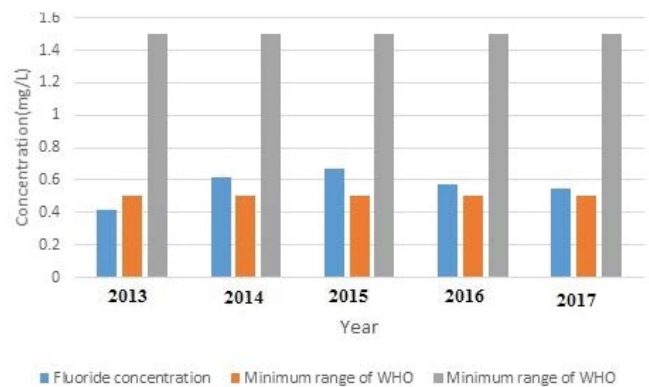
Fig. 2. Comparison of annual mean fluoride concentrations in the studied area with WHO guideline of fluoride in drinking water.
