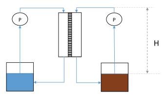
Fig. 3. Considered pumping arrangement for circulation energy requirement calculation.
