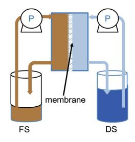
Fig. 1. Experimental layout.
