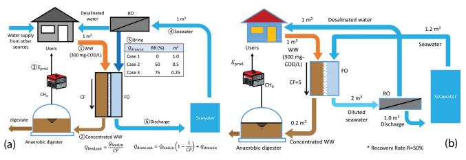
Fig. 2. Two different scenarios considered in this study: (a) FO following RO and (b) RO following FO.
