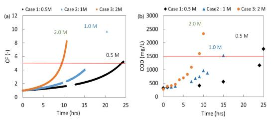
Fig. 4. Results of the FO process for wastewater concentration using different concentrations for the draw solution. (a) Concentration factor, (b) COD concentration levels.
