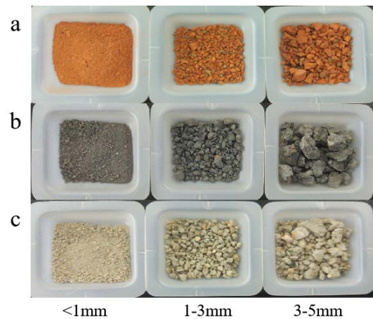
Fig. 1. Photographs of selected C & D bricks: (a) red bricks, (b) concrete blocks, and (c) burn-free bricks.
