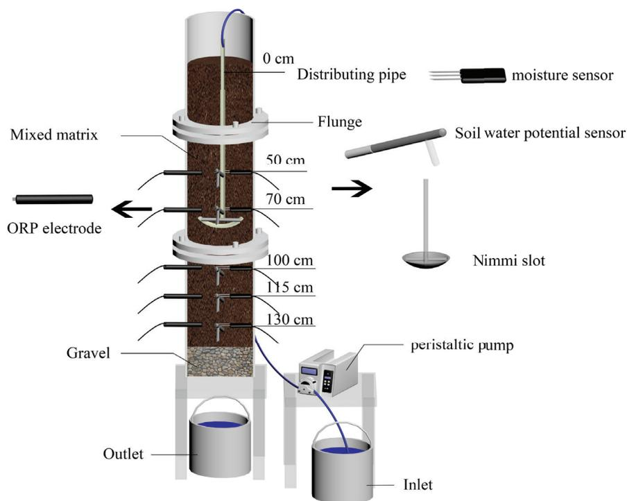
Fig. 1. Schematic diagram of the SWIS. A peristaltic pump (Prefluid BT100 - YZ15) controls the hydraulic load ( $0.10 \text{ m}^3 \cdot (\text{m}^2 \cdot \text{d})^{-1}$ ). A transmitter (MDAS) which was connected with all the probes was invented by Nanjing Soil Research Institute. The computer was utilized to accept data.
