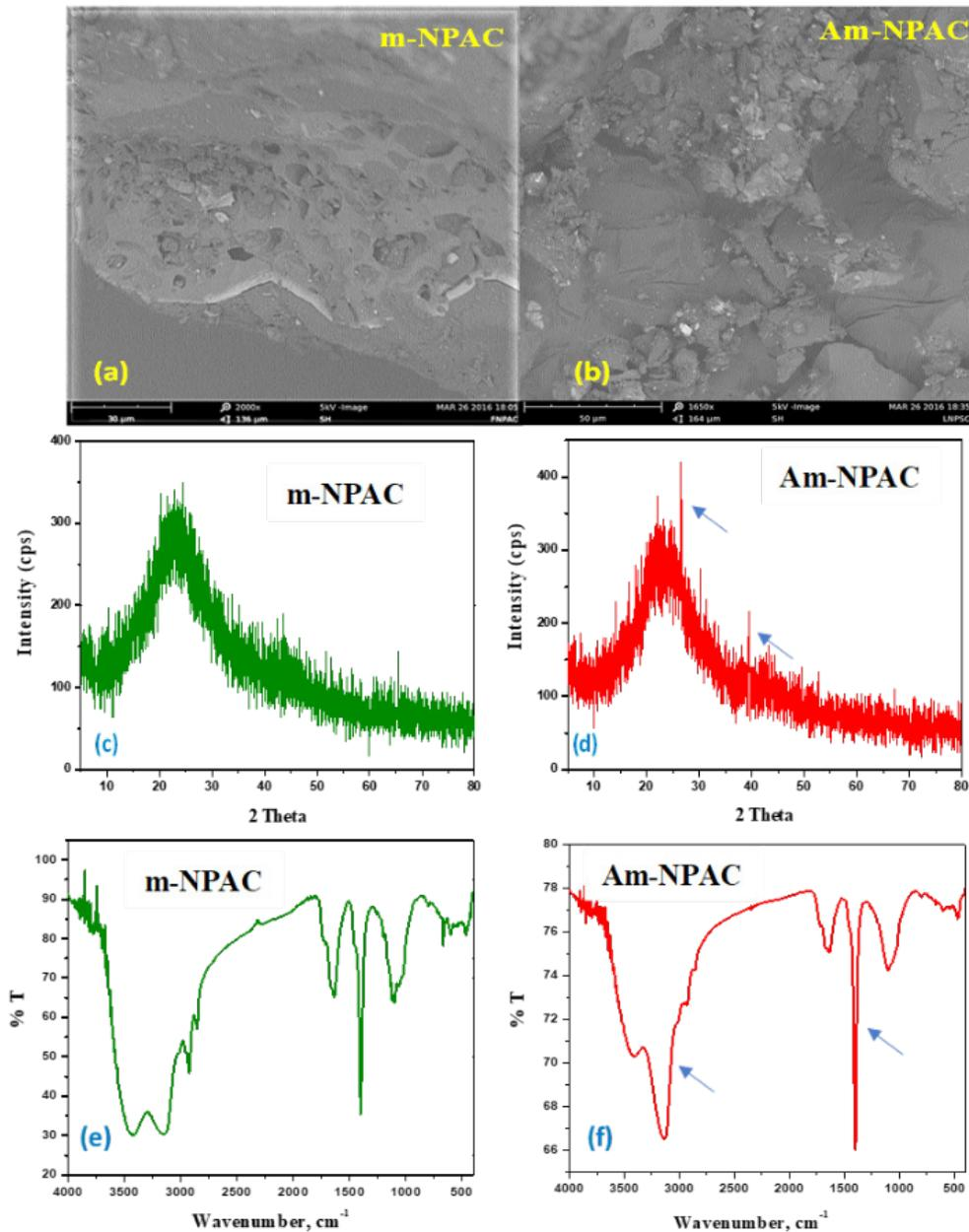
Fig. 4. (a, b) SEM, (c, d) images, XRD spectra and (e, f) FT-IR spectra of (a) m-NPAC and (b) Am-NPAC.
