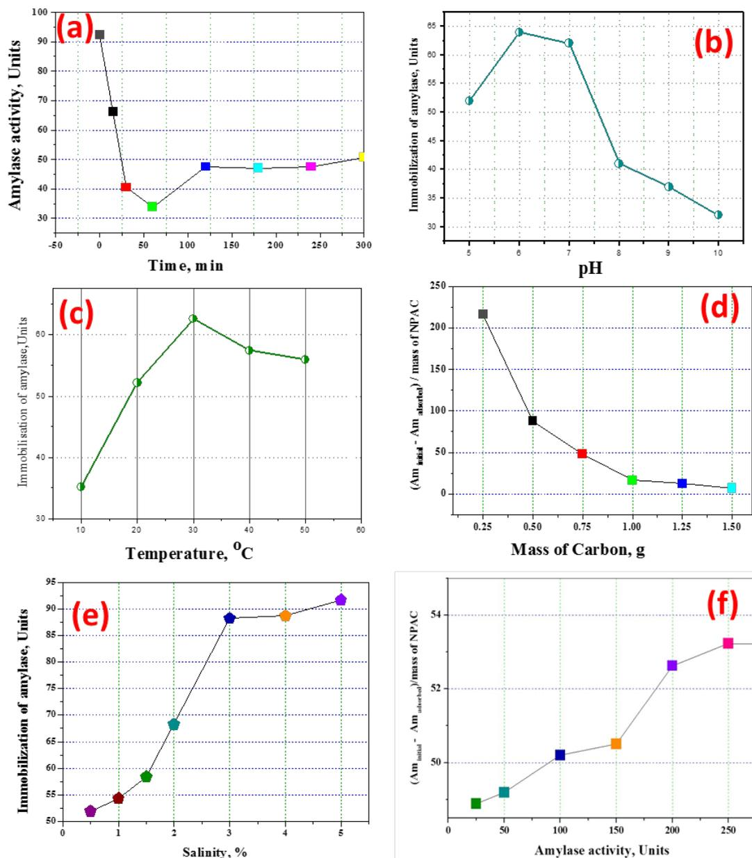
Fig. S1. Optimization studies on the effect of (a) time (b) pH (c) temperature (d) mass of carbon (e) salinity and (f) amylase concentration on the immobilization of amylase onto m-NPAC.
