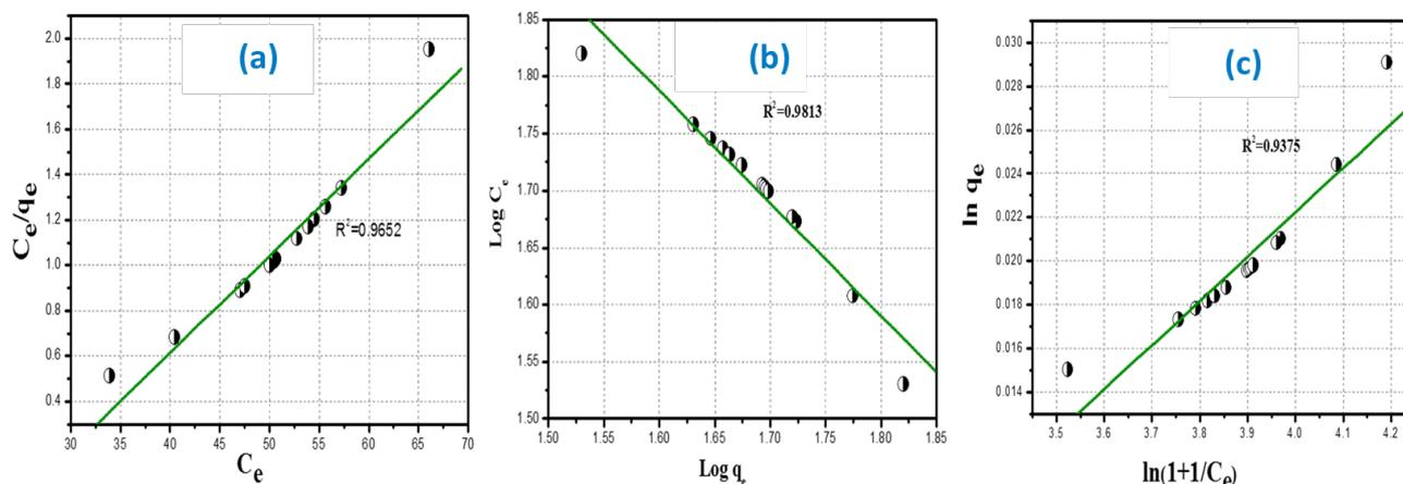
Fig. 5. (a) Langmuir (b) Freundlich and (c) Dubnin-Radushkevitch adsorption isotherm models for the immobilisation of saline tolerant amylase onto the surface of m-NPAC.
