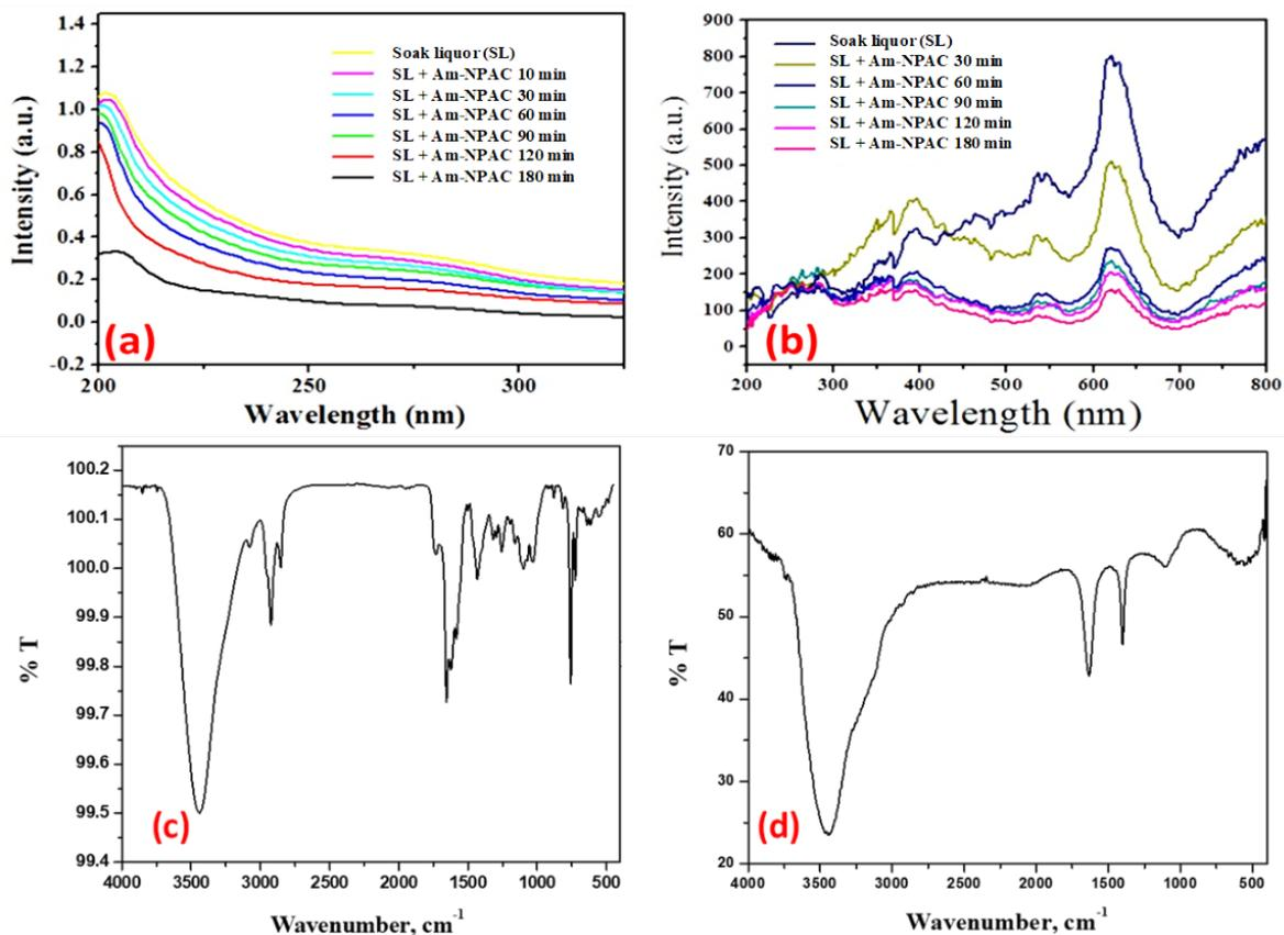
Fig. 9. (a) UV-visible and (b) UV-fluorescence spectra and (c) FT-IR spectra of degraded mucopolysaccharide contents of soak liquor using Am-NPAC.
