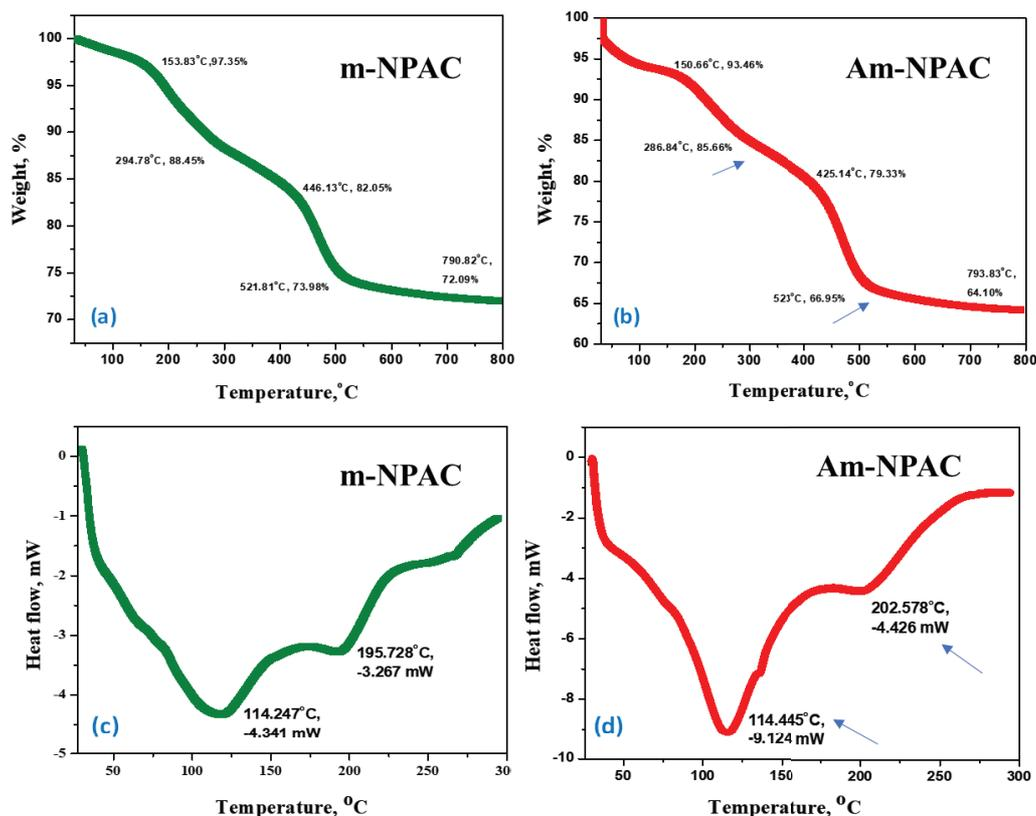
Fig. 3. (a, b) TGA and (c, d) DSC spectra of m-NPAC and Am-NPAC.
