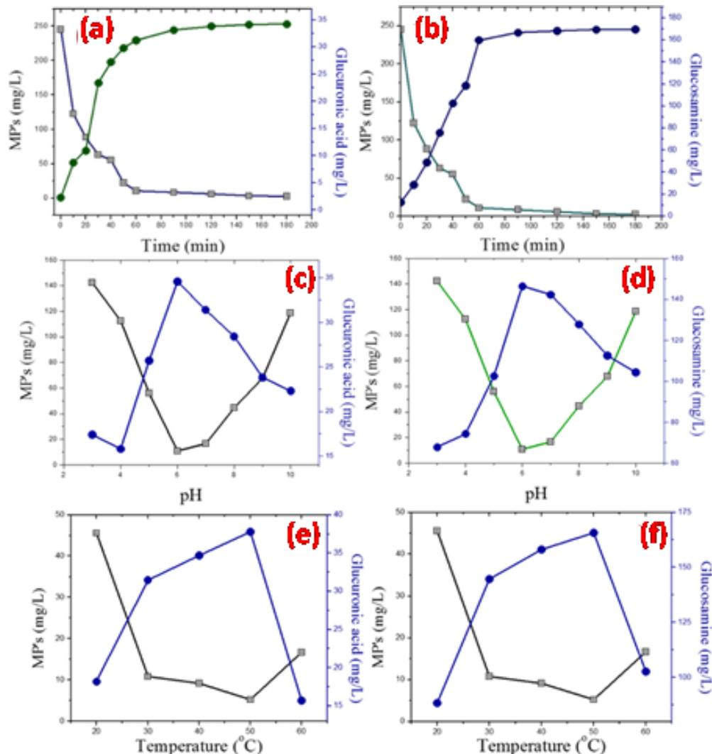
Fig. 6. Optimization of (a, b) time (c, d) pH and (e, f) temperature for the degradation of mucopolysaccharides content of soak liquor concerning the formation of (a) glucuronic acid and (b) glucosamine.
