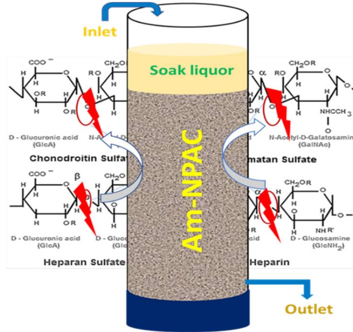
Fig. 7. Schematic representation of the degradation of mucopolysaccharides of soak liquor using Am-NPAC packed bed reactor.
