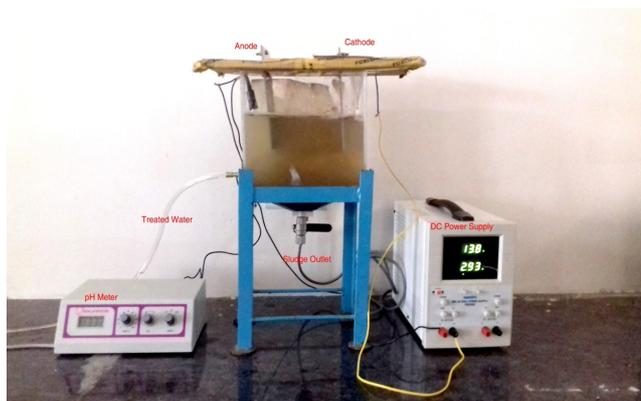
Fig. 1. Experimental setup of electro-chemical peroxidation reactor.
