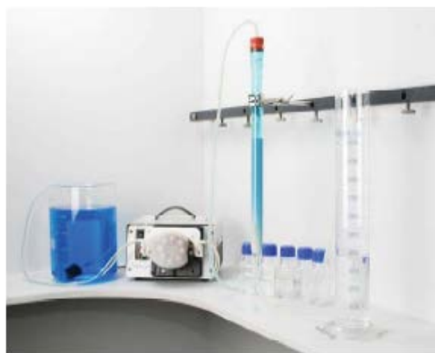
Fig. 1. Experimental set-up for the ion-exchange treatment process.
