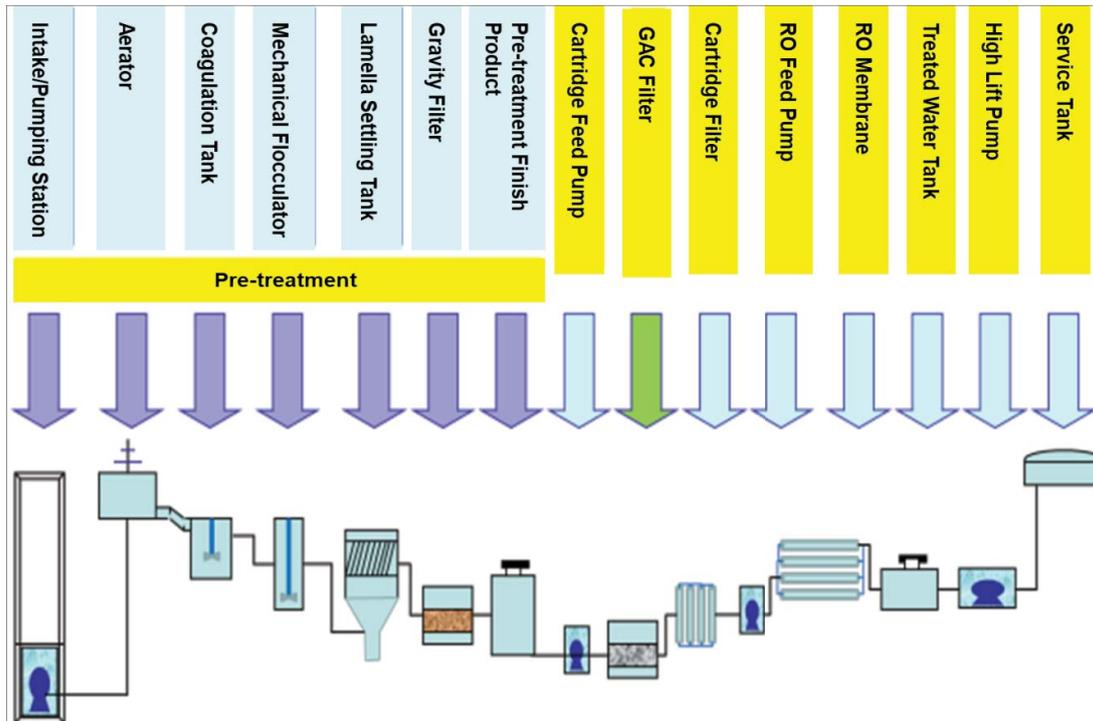
Fig. 2. Treatment plant arrangement.
