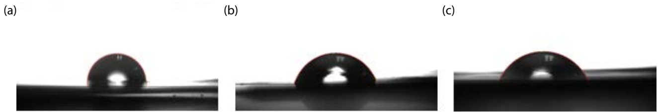
Fig. 6. Contact angle and liquid entry pressure for membranes exposed to ultrasonic irradiation at different frequencies (a) 28 kHz, 30 W; (b) 45 kHz, 30 W; and (c) 72 kHz, 300 W.
