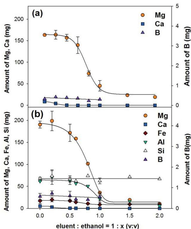
Fig. 9. Amount of components remaining in the filtrate after  $MgSO_4$  precipitation depending on the volume ratio of eluent to ethanol (a) 1.0 M eluent and (b) 1.5 M eluent.
