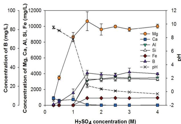
Fig. 6. Concentrations of Mg, Ca, Al, Si, Fe, and B and the pH of the eluent depending on the concentration of  $\text{H}_2\text{SO}_4$ .
