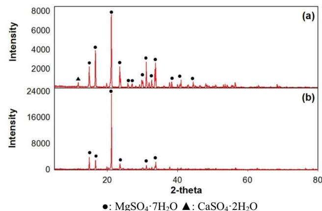
Fig. 10. X-ray diffraction results of the precipitated  $MgSO_4$  when the ratio of eluent to ethanol was 1:1: (a) 1.0 M eluent and (b) 1.5 M eluent.
