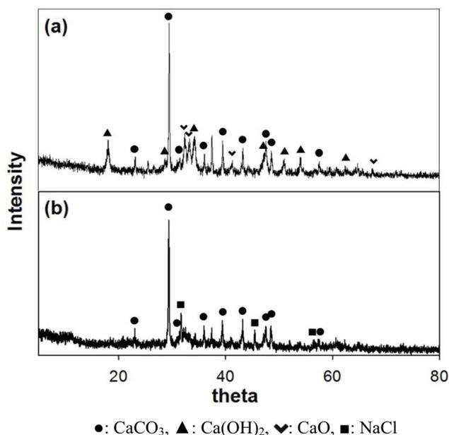
Fig. 5. X-ray diffraction results: (a) raw paper sludge ash (PSA) and (b) solid obtained after filtering the mixture of PSA and brine when the ratio was 1:40.
