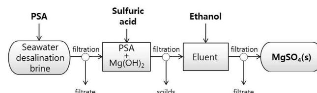
Fig. 2. Three-step process for recovering Mg from seawater desalination brine.
