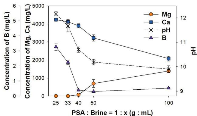
Fig. 4. Concentrations of Mg, Ca, and B and the pH of the filtrate depending on the ratio of paper sludge ash (PSA) to brine.
