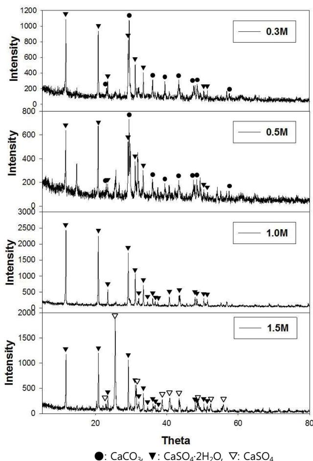
Fig. 7. X-ray diffraction results of solids remaining after dissolving Mg with 0.3–1.5 M  $\text{H}_2\text{SO}_4$ .
