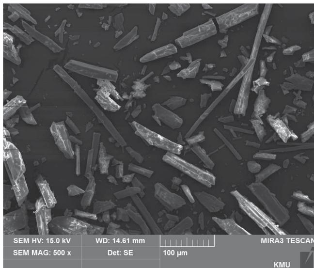
Fig. 11. Scanning electron microscope (SEM) image of the precipitated  $\text{MgSO}_4$  using 1.0 M eluent when the ratio of eluent to ethanol was 1:1.
