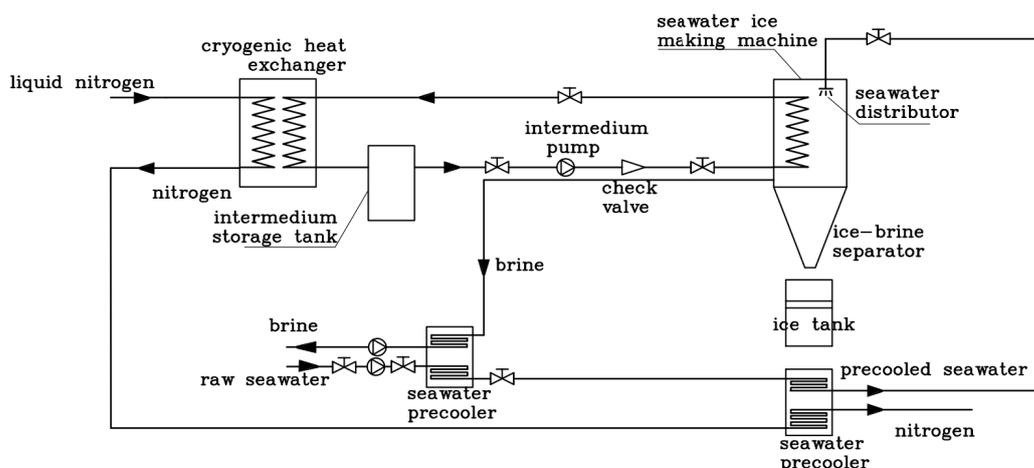
Fig. 2. Flow diagram of the platform.
