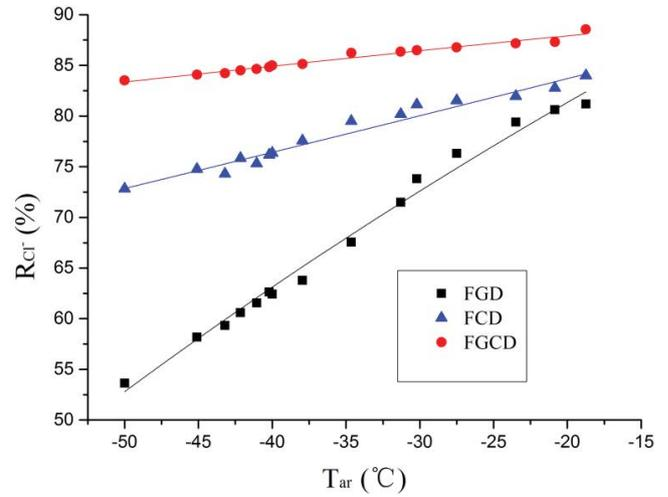
Fig. 10. Relationships between  $R_{Cl^-}$  and  $T_{ar}$  for FGD, FCD and FGCD processes.
