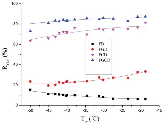
Fig. 8. Relationships between  $R_{TDS}$  and  $T_{ar}$  for FD, FGD, FCD and FGCD processes.
