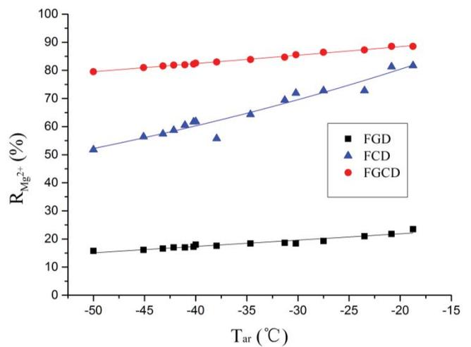
Fig. 12. Relationships between  $R_{Mg^{2+}}$  and  $T_{ar}$  for FGD, FCD and FGCD processes.
