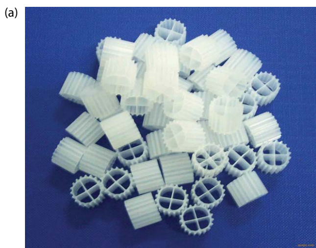
Fig. 1. Physical images of YL-1 (a) and YL-2 (b) suspended carriers.
