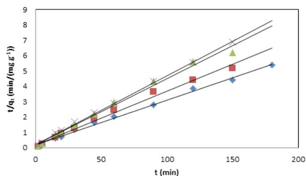
Fig. 5. The fitting of pseudo-second-order model for the adsorption of phenol onto the [poly(EGDMA-VIM)] microspheres (phenol concentration of 60 mg L<sup>-1</sup>, natural pH, adsorbent dosage of 50 mg g<sup>-1</sup>) (♦ 25°C ■ 35°C ▲ 45°C × 55°C).
