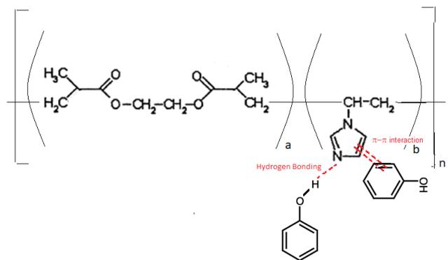
Fig. 9. Possible interactions between the *[poly(EGDMA-VIM)]* microspheres and the phenol.
