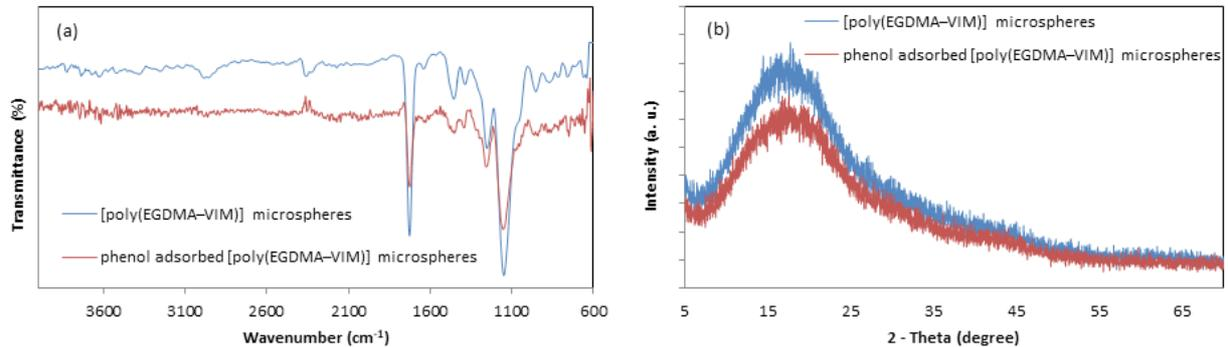
Fig. 7 (a) FTIR spectrum (b) XRD patterns for the *[poly(EGDMA-VIM)]* microspheres before and after adsorption of phenol.
