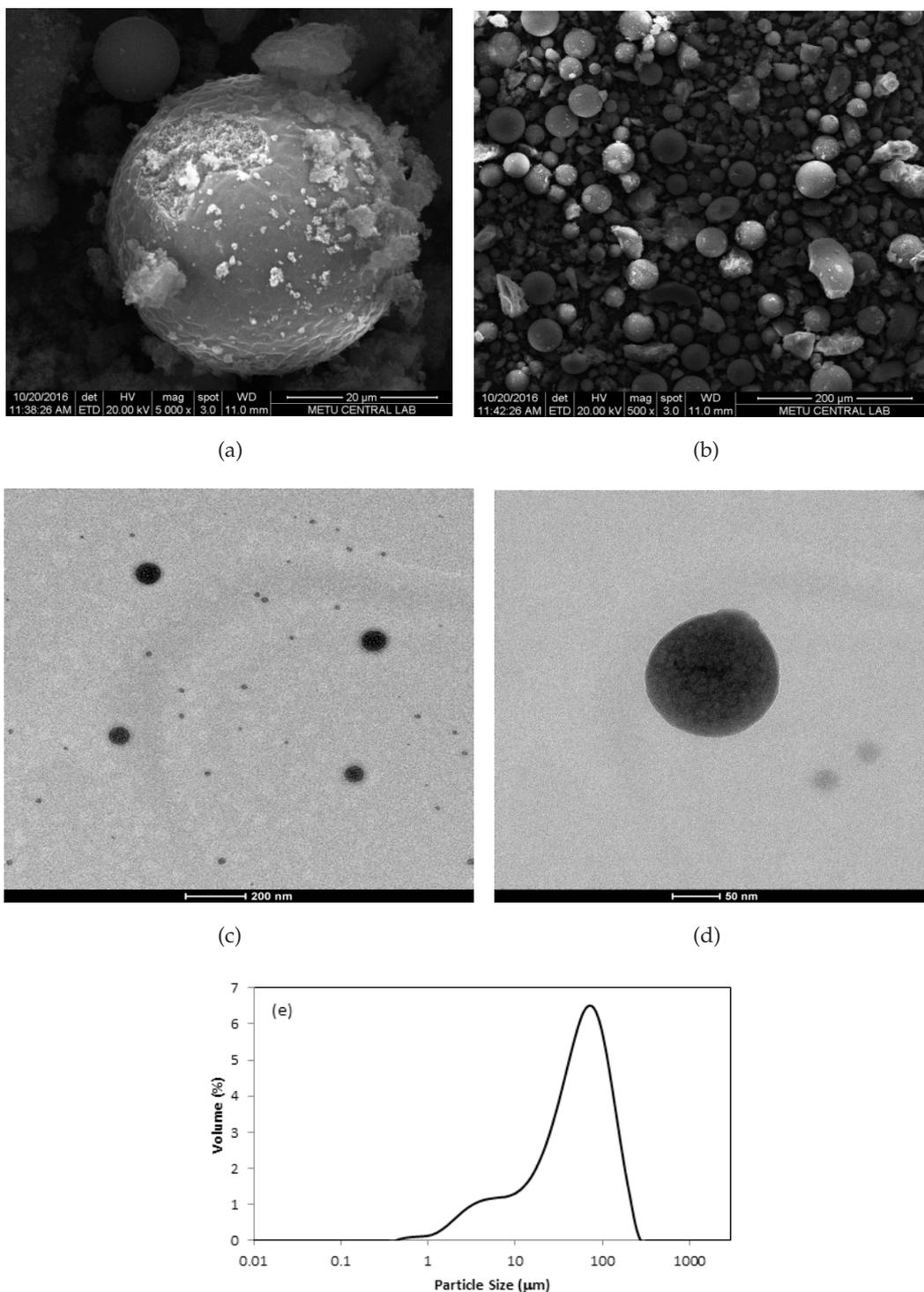
Fig. 3. SEM micrographs (a) 20  $\mu\text{m}$  (b) 200  $\mu\text{m}$ , TEM images (c) 200 nm (d) 50 nm, (e) the particle size distribution for the *[poly(EGDMA-VIM)]* microspheres.
