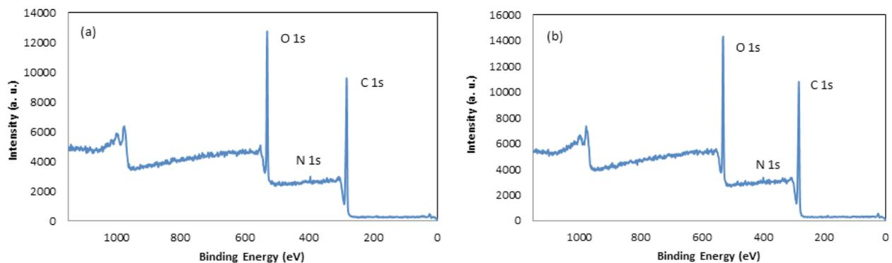
Fig. 8. XPS energy spectra of the *[poly(EGDMA-VIM)]* microspheres (a) before and (b) after phenol adsorption.
