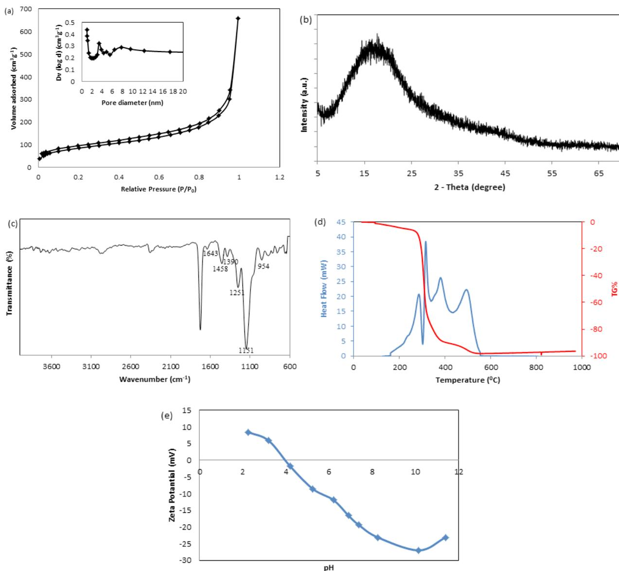
Fig. 2. (a) N<sub>2</sub> adsorption-desorption isotherm and pore-size distribution (inset) (b) XRD pattern (c) FTIR spectra (d) TGA and DTA curves (e) Zeta potential of the *[poly(EGDMA-VIM)]* microspheres.
