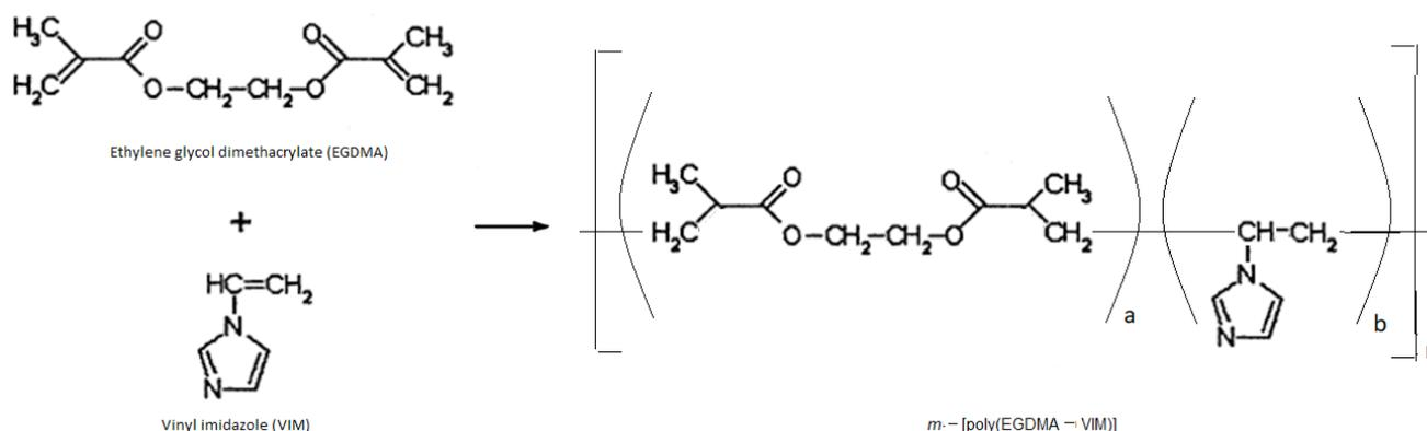
Fig. 1. Polymerization scheme for the preparation of the  $[poly(EGDMA-VIM)]$  microspheres [32].
