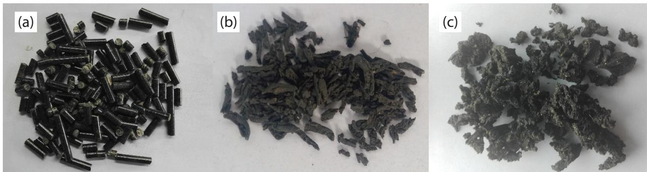
Fig. 2. Feedstocks of dried SS prior to the MP process (a) pelletized SS with additive; (b) noodle shape without additive; (c) lump shape without additive.
