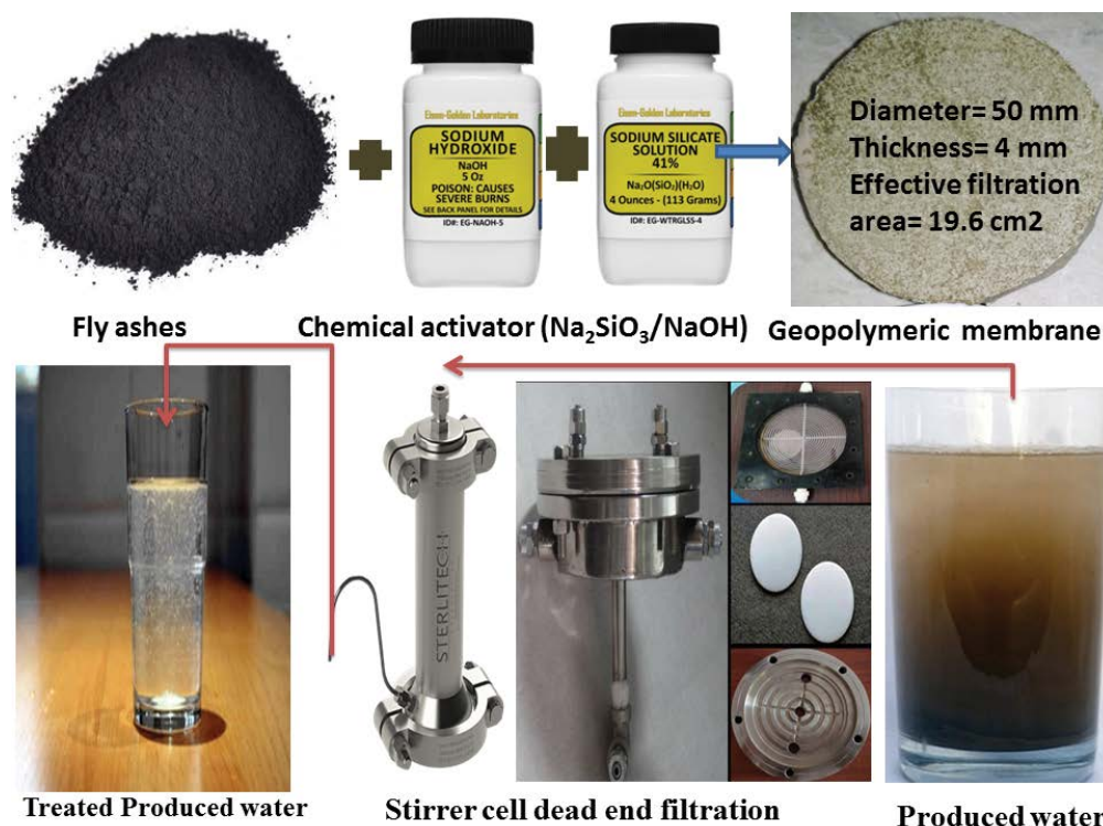
Fig. 1. Synthesis of geopolymeric membrane for produced water treatment.
