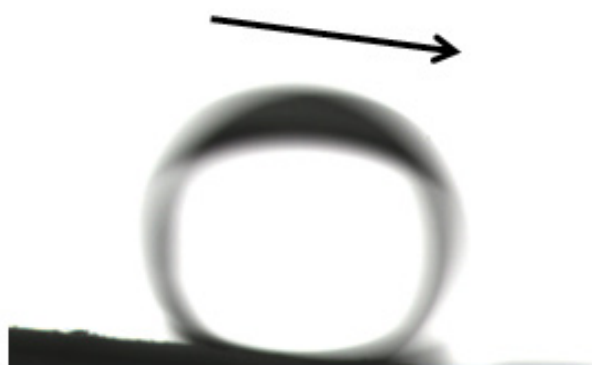
Fig. S4. A typical image of an oil droplet slides away from the surface of the Ca-ALG/Ag hydrogel film (5 μL, 1, 2-dichloroethane).
